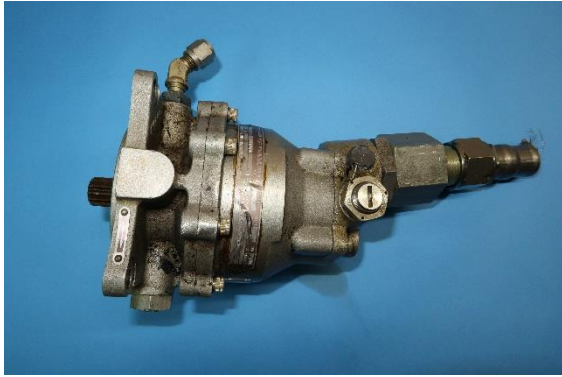
Figure 11. Hydraulic pump after removal from the transmission.
