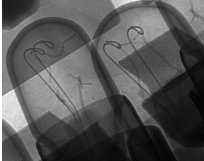
Figure 22. Radiograph showing broken and unstretched filaments of the HYD PRESS lightbulbs.
