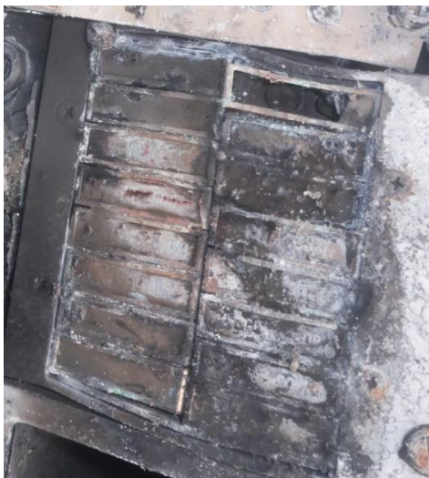
Figure 20. Caution panel as found installed in the instrument panel.
