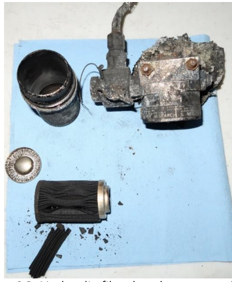
Figure 14. Hydraulic filter bowl unscrewed from the assembly and the filter element removed from the bowl.
