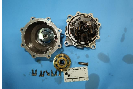
Figure 12. Hydraulic pump disassembly.
