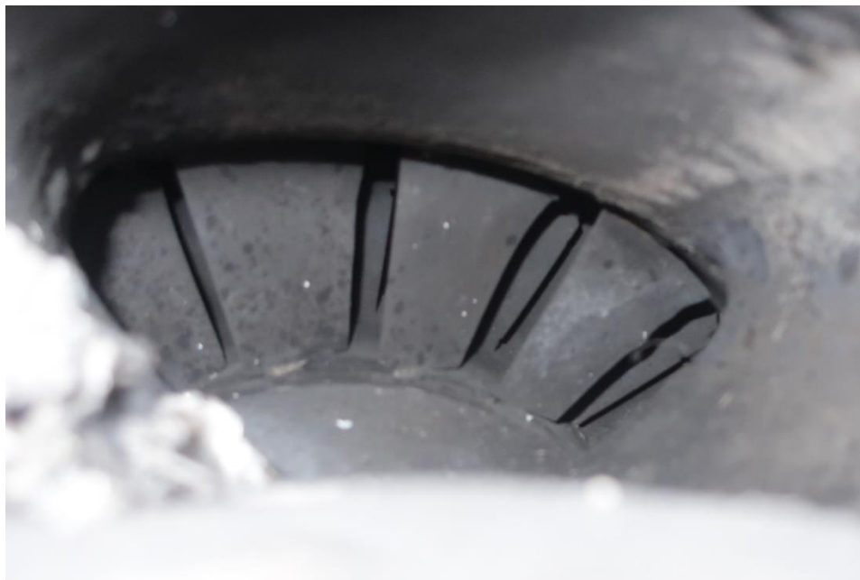
Figure 9. Compressor inlet, a section of the first stage compressor blades visible.
