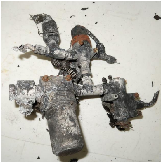
Figure 13. Filter with attached pressure switch.
