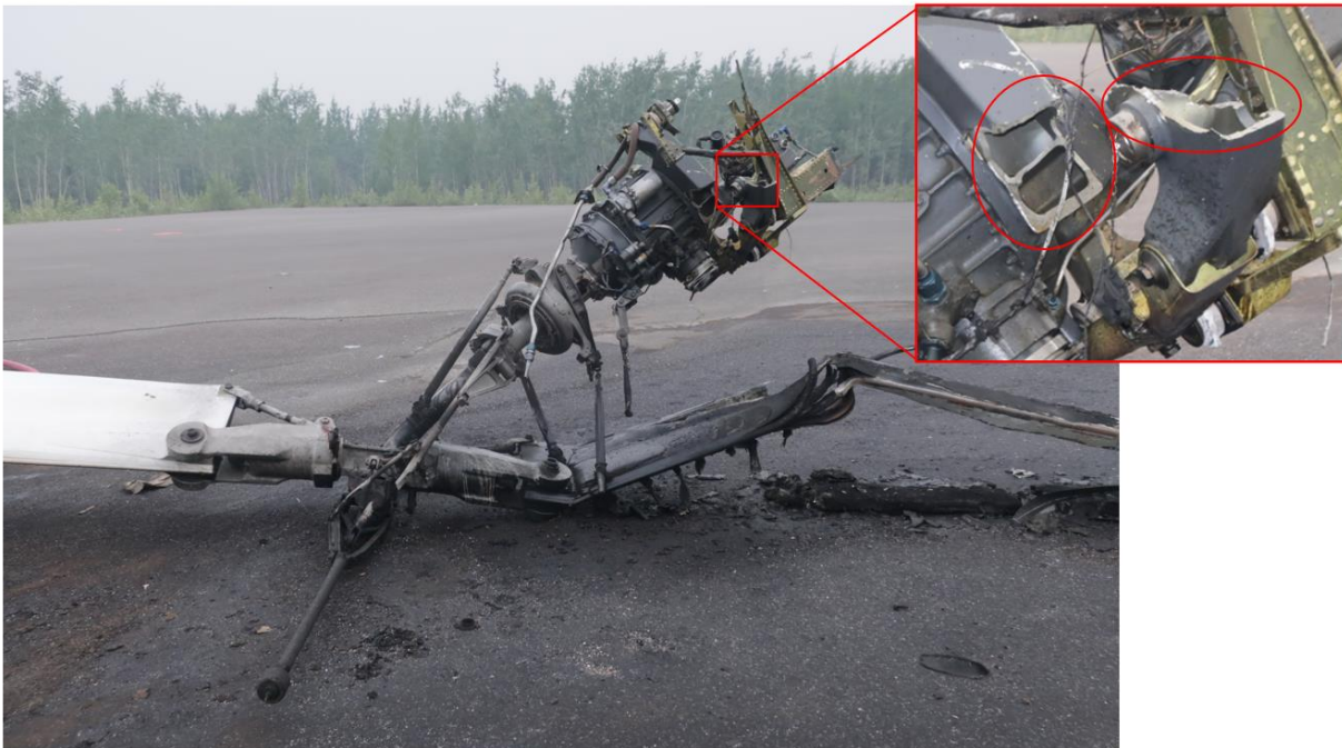
Figure 3. Main rotor and transmission. Transmission support case fracture shown in the red inset box.
