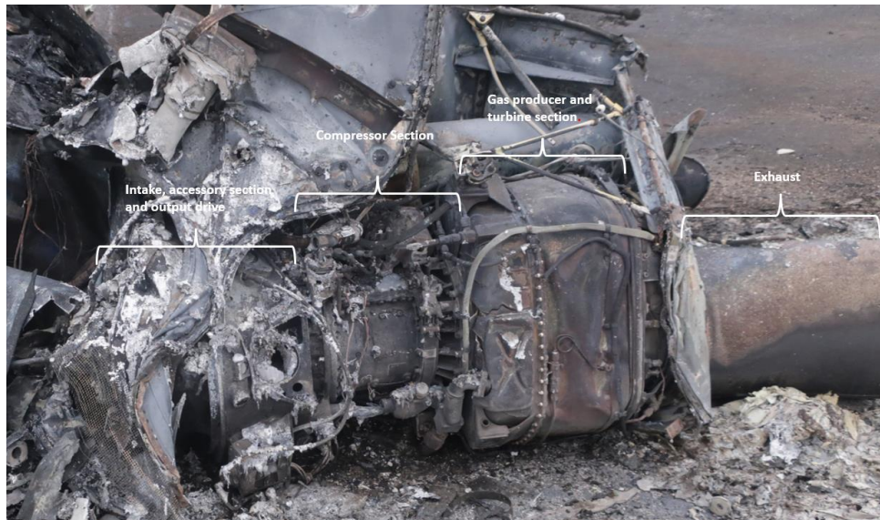
Figure 8. The engine as found in the wreckage.
