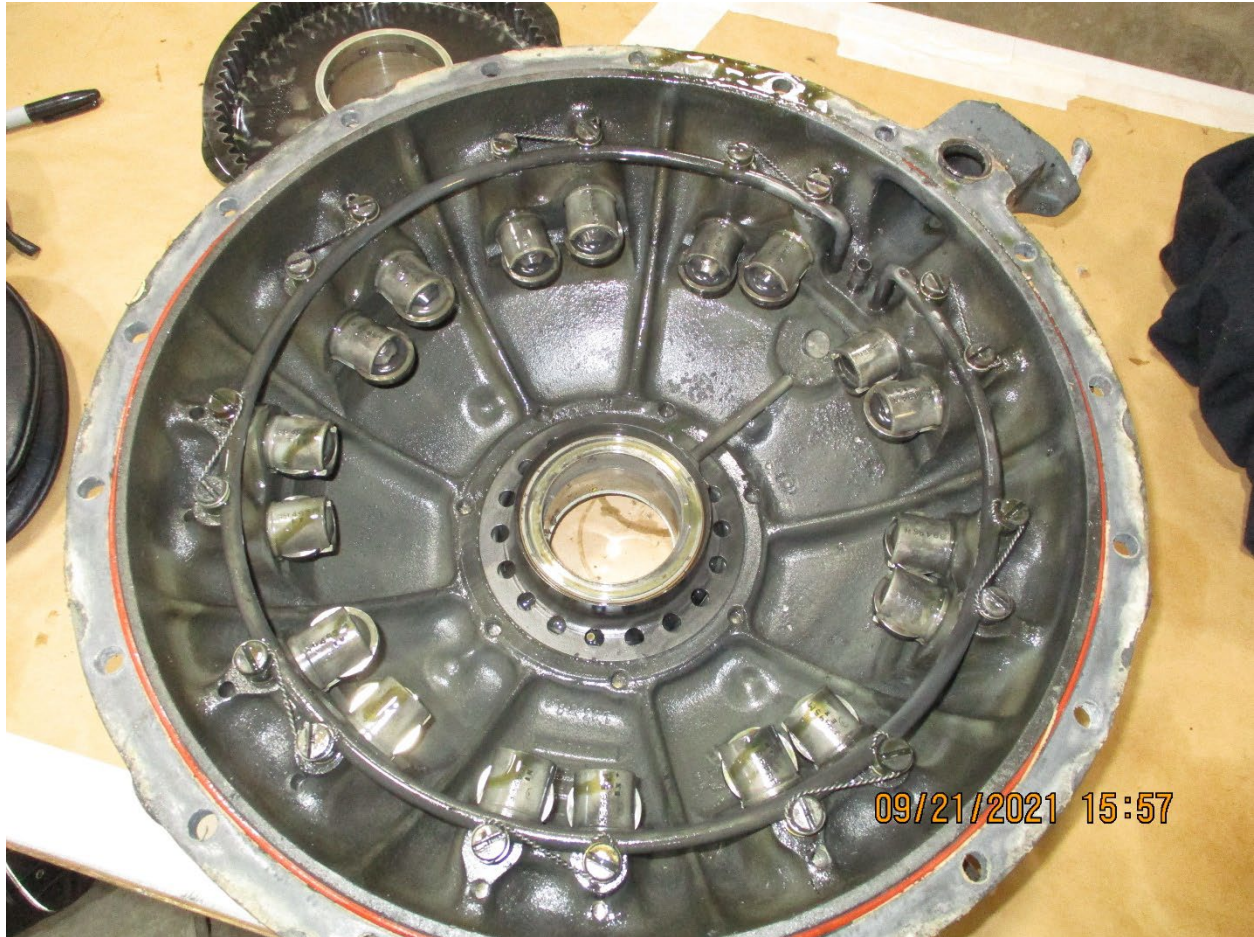
Figure 8. View of lifters and rollers inside of nose cone.
