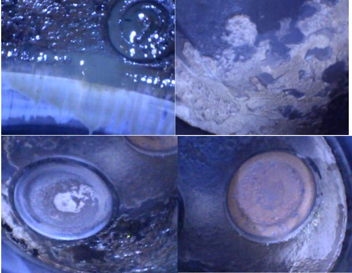
Figure 25. Cylinder No. 4 Spark plug, Piston, Top, Intake Valve, and Exhaust Valve.
