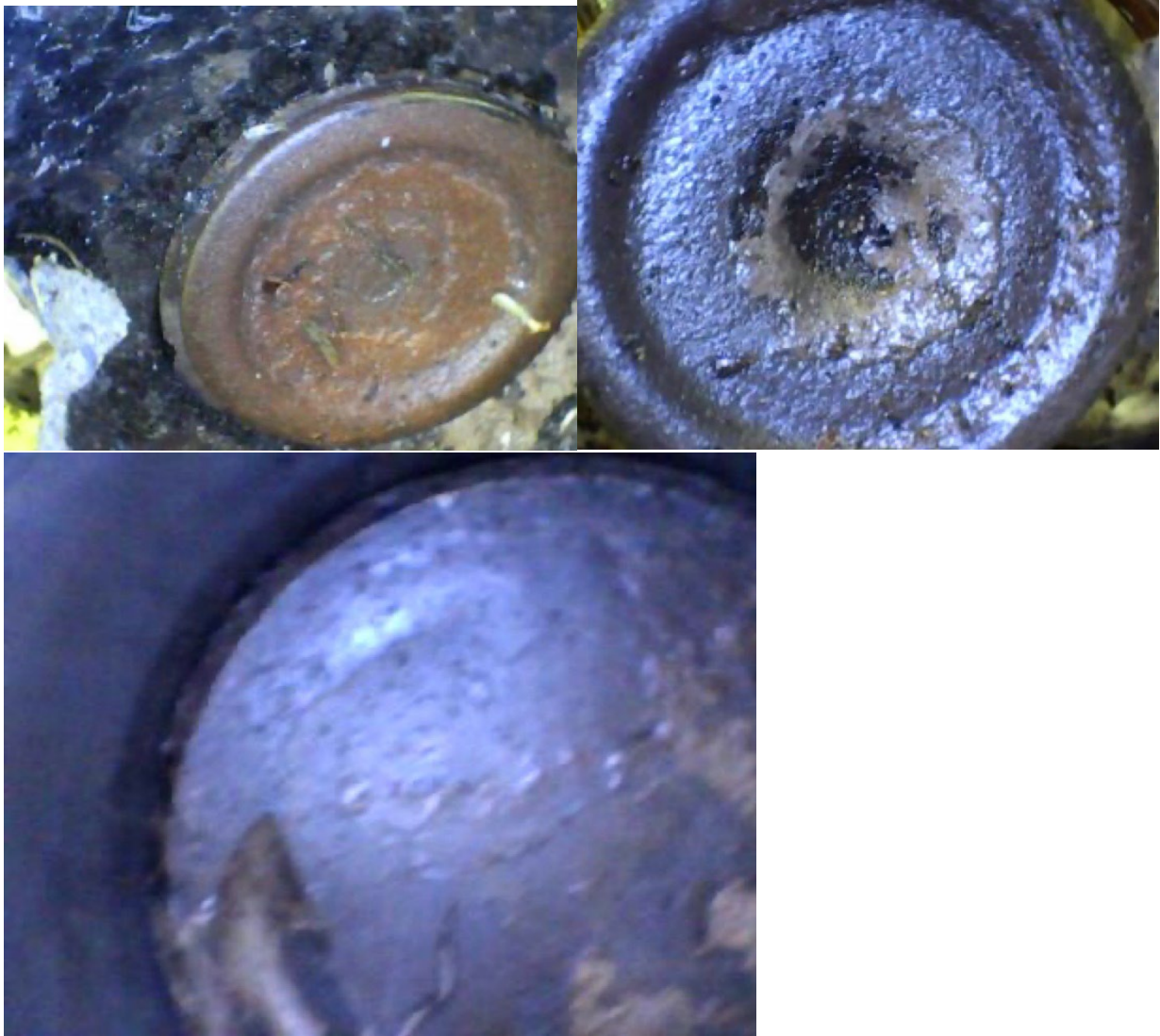
Figure 27. Cylinder No. 6 Exhaust Valve, Intake Valve, and Piston Top
