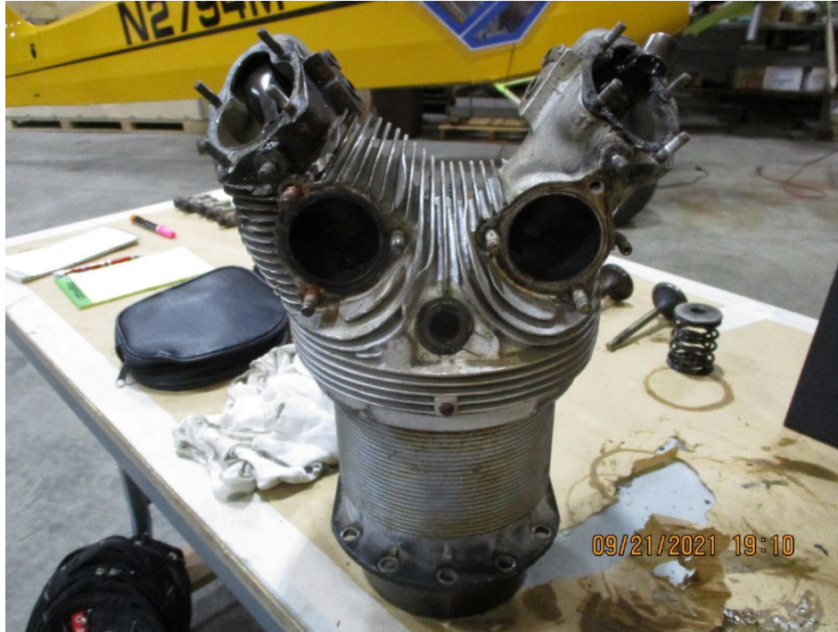
Figure 11. No. 1 cylinder after removal.
