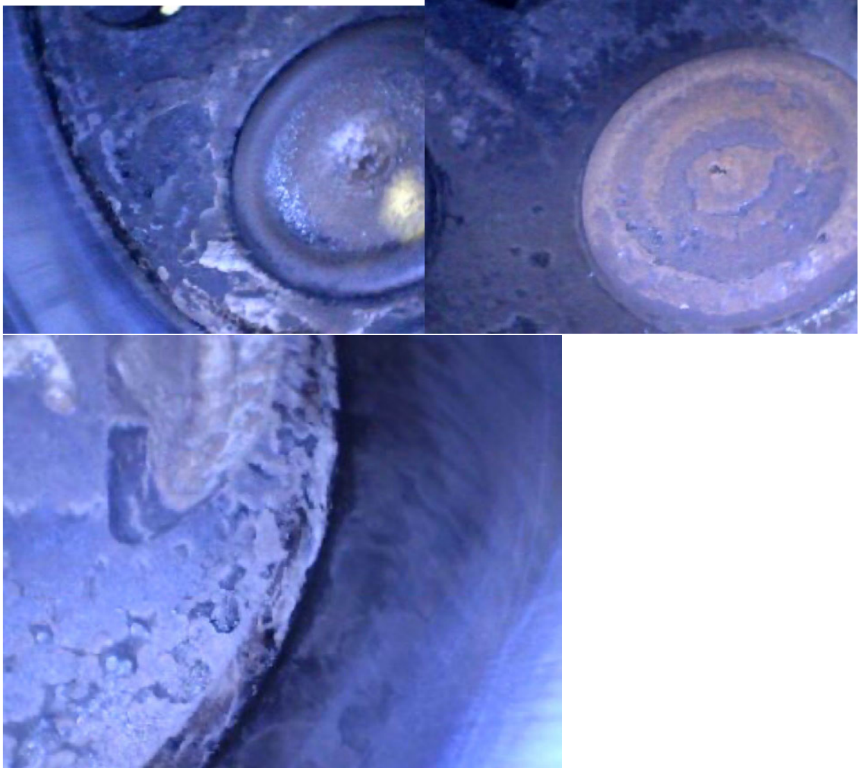
Figure 24. Cylinder No. 3 Intake Valve, Exhaust Valve, Piston Top, and Cylinder Wall
