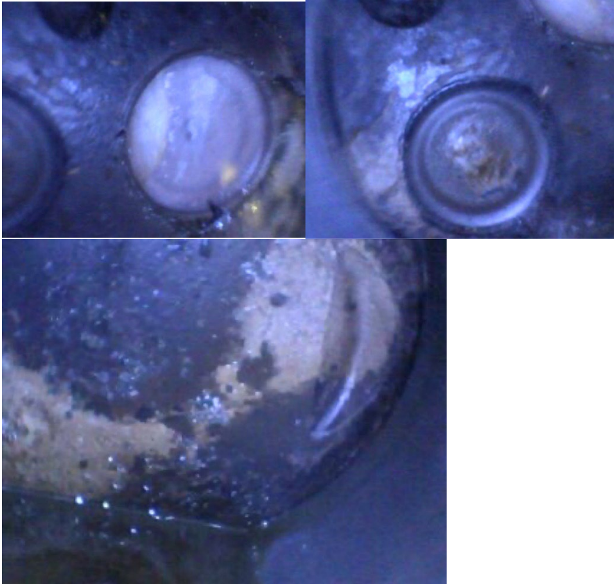
Figure 29. Cylinder No. 8 Exhaust Valve, Intake Valve, and Piston Top. Note oil in the cylinder.
