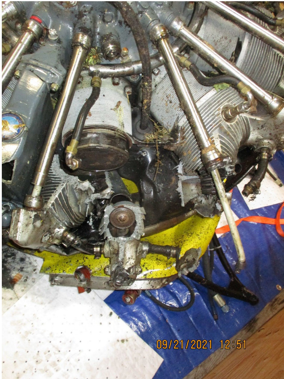
Figure 3. View of Nos. 6 & 7 cylinder damage. Note tree debris in cylinder fins.
