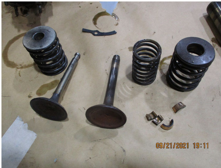
Figure 14. No. 1 intake valve, exhaust valve, springs, and keepers.
