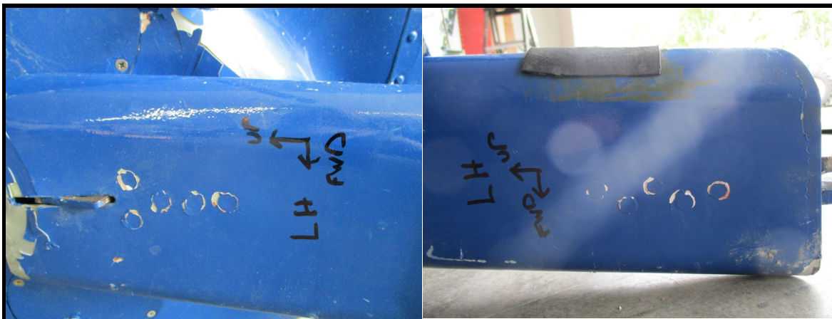
Figure 3-Left wing strut, lower surface, upper (left) and lower (right) strut fitting rivets.
