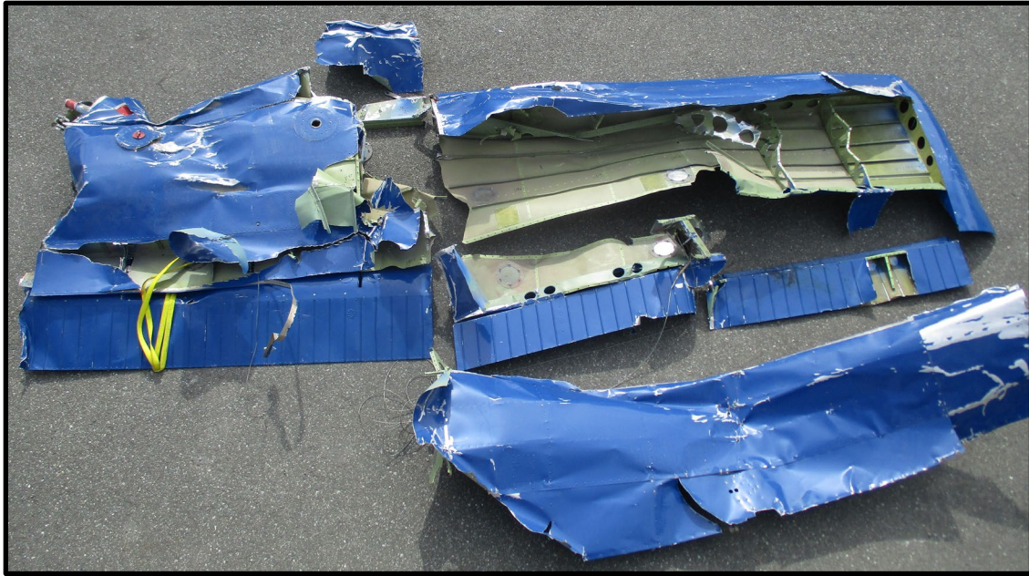
Figure 4-Right wing wreckage layout (strut not shown).
