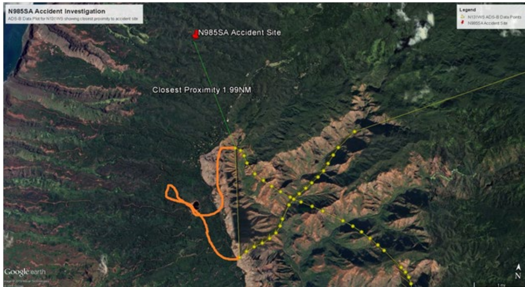
Figure 6: Accident location and ADS-B track of Sunshine Helicopters. The orange track was drawn by the Sunshine Helicopters pilot to estimate his ground track in an area that lacked ADS-B coverage.
