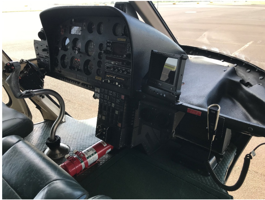
Figure 10: Supplemental type certificate modification to flight controls in N702SA.
