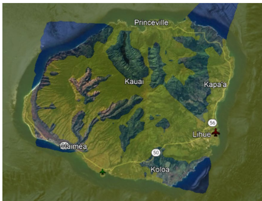
Figure 16. ADS-B service for aircraft at 500 feet agl or higher, above or near Kauai.
