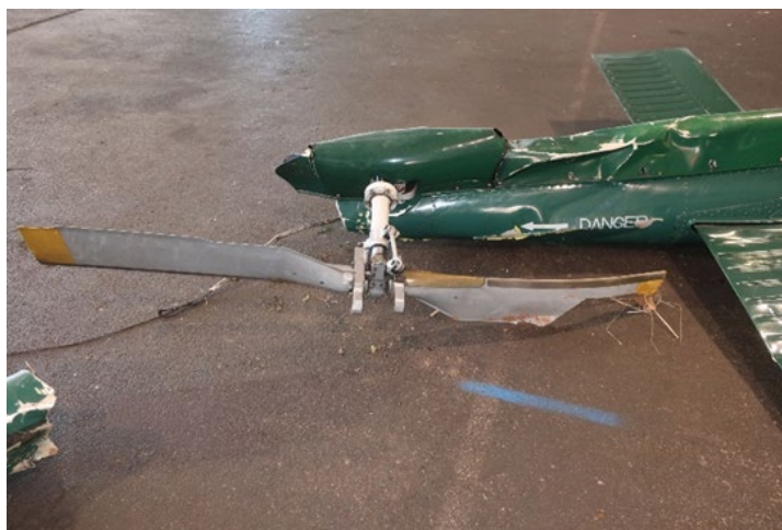
Photo 11 – Tail rotor blades remained attached to the hub and gearbox.
