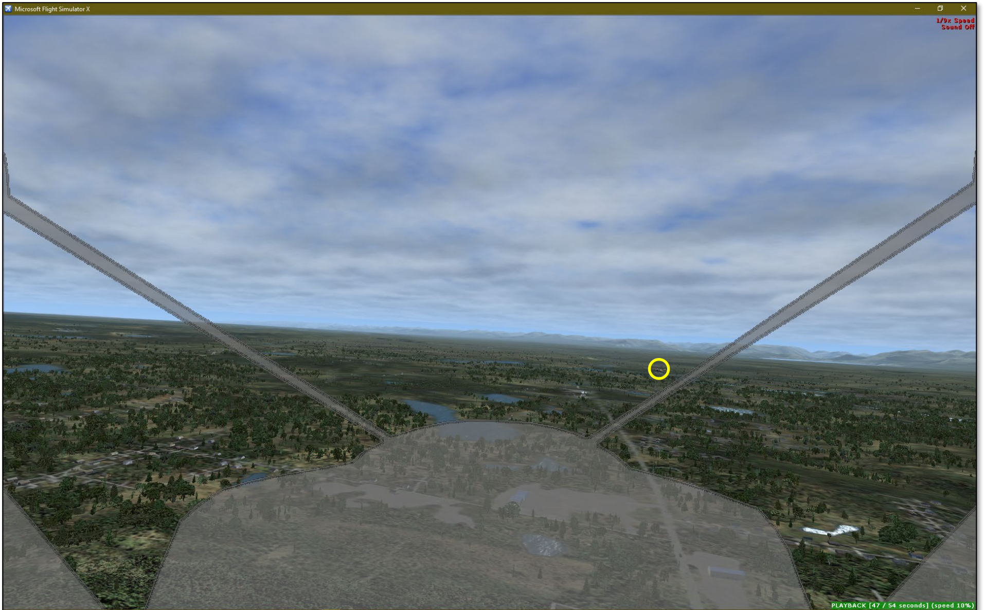
Figure 15f. Recreation of the view from the Piper cockpit at 08:26:27 (5.3 seconds before the collision). The location of the Beaver is indicated by the yellow circle.
