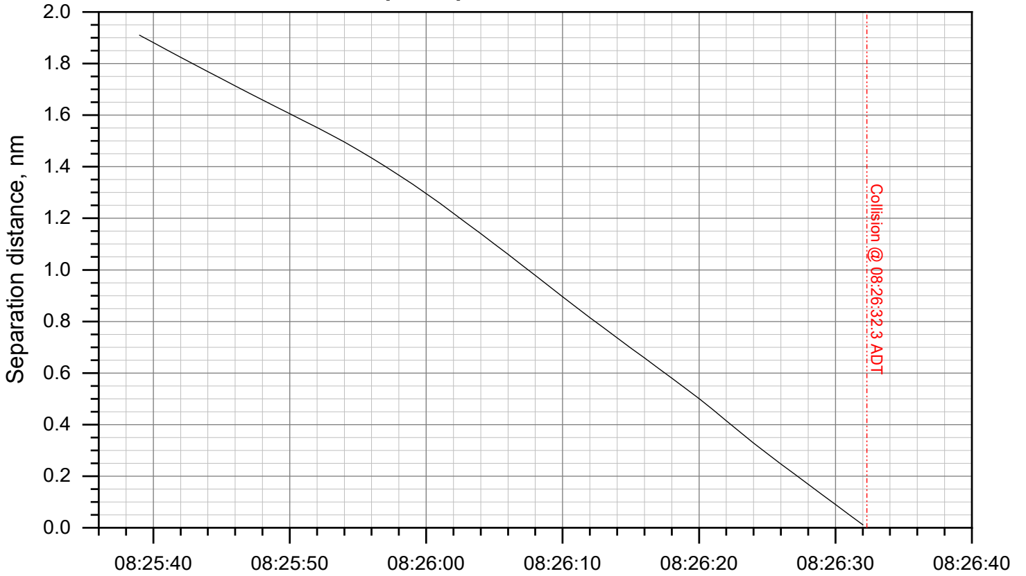
Beaver and Piper separation distance and closure rate
