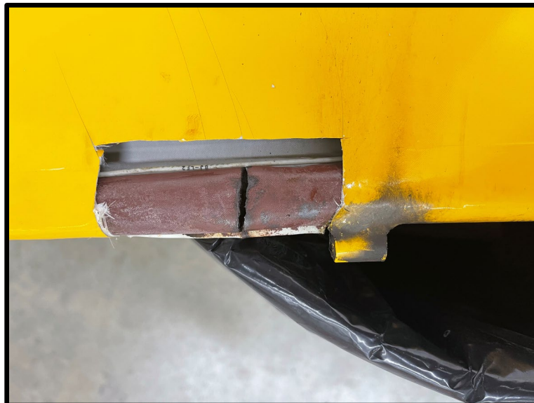
Figure 2-PA-18 fractured rudder post.
