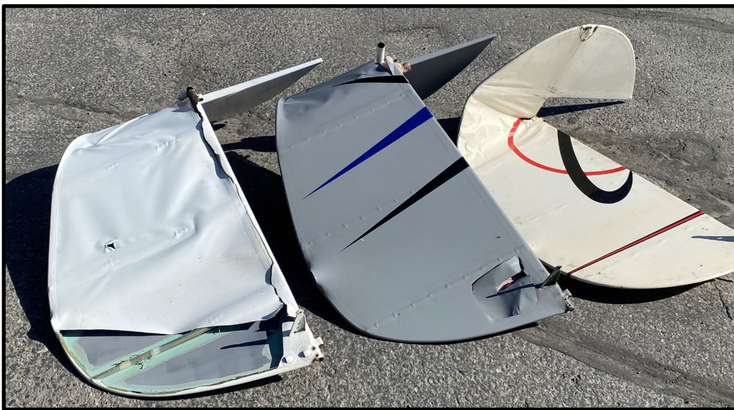
Figure 1-PA-12 fractured rudders; grey rudder is from accident airplane.
