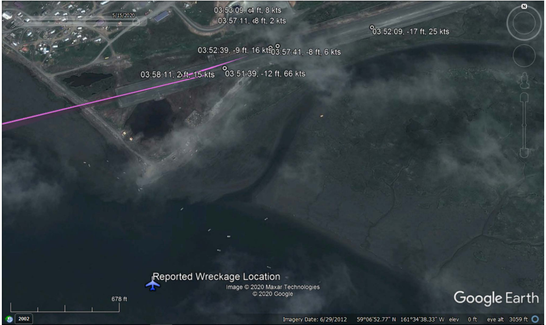
Figure 4. Google Earth overlay of the end of the last session recorded on the Garmin Aera 796.
