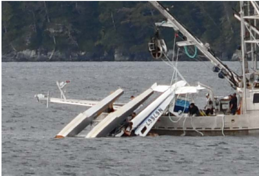
Figure 2. Rescue boat pulling airplane out of water with ropes around empennage
