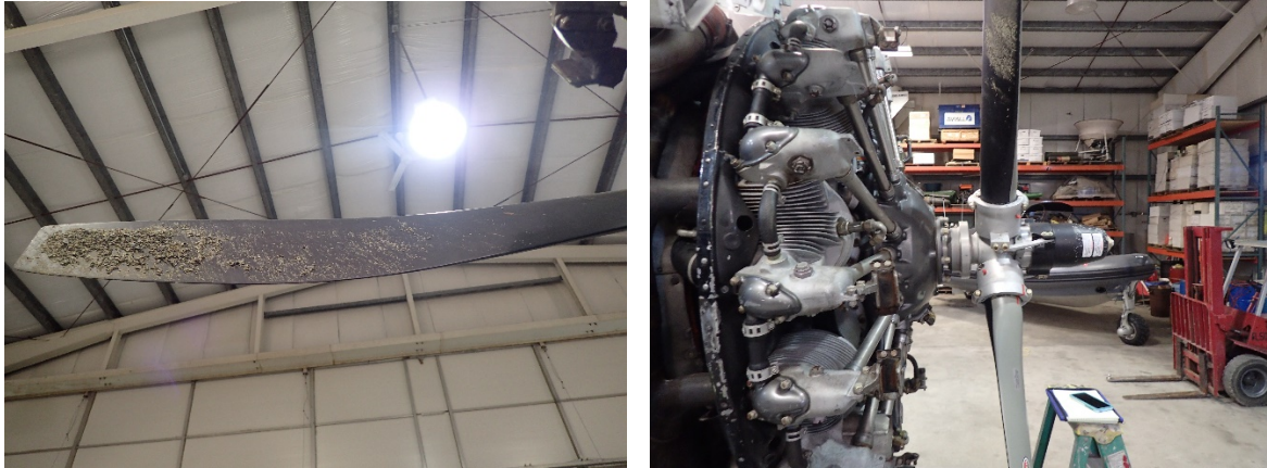
Figure 10. Hartzell propeller and blade “A” with mild bend
