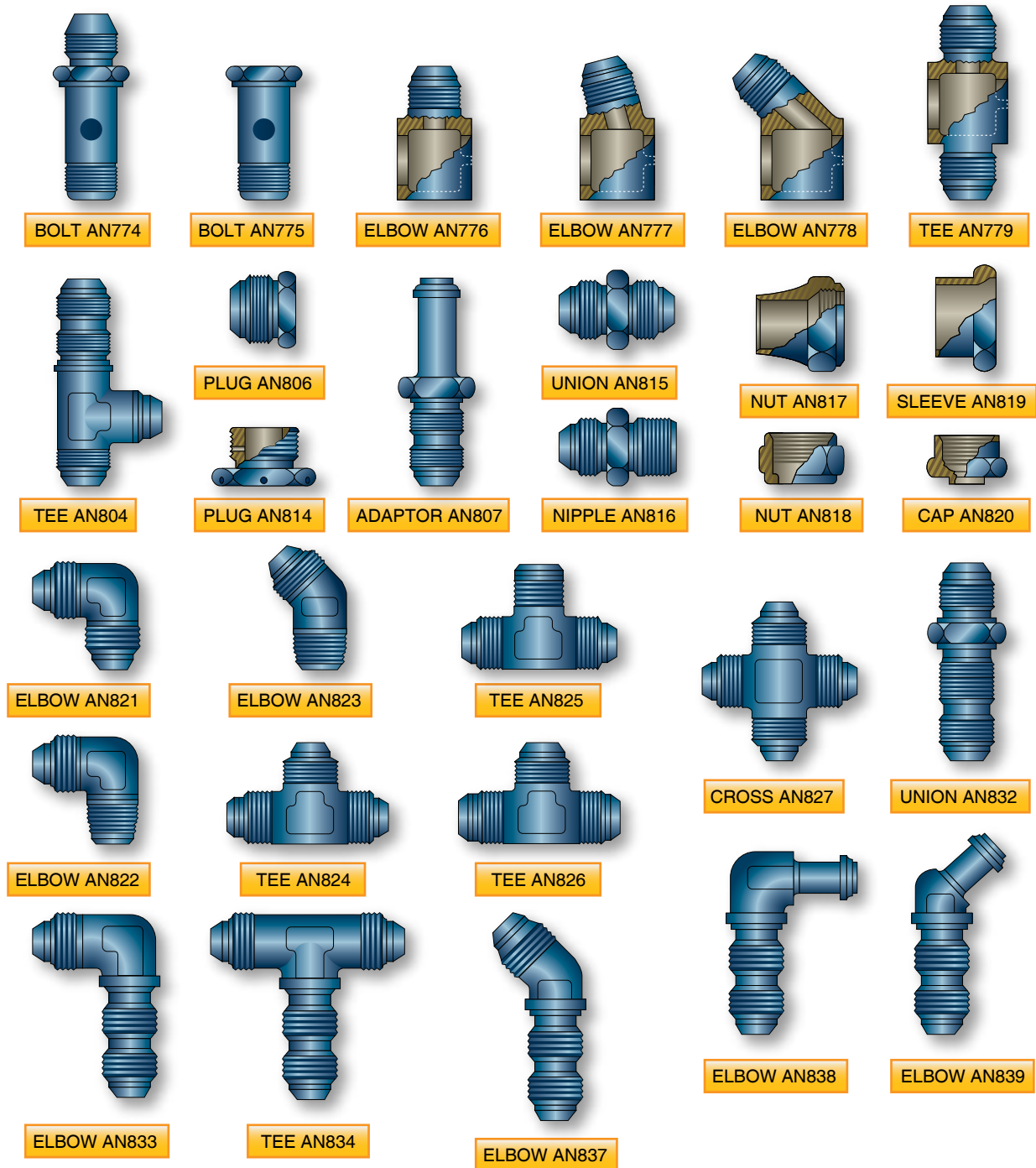
Figure 9-19. AN standard fittings.
