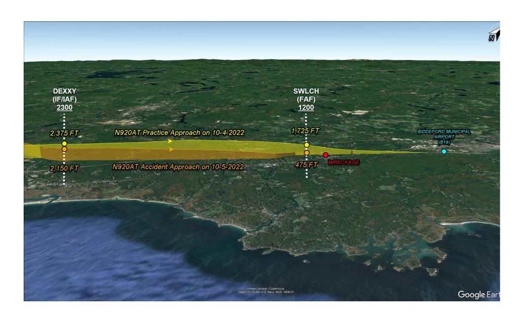
Photo 3 – Accident Track Superimposed over Practice Approach of Previous Day (NTSB)
