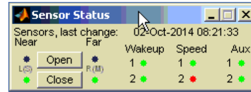
Sensor status window from RailBAM® web page and GUI, showing 'Speed Sensor 2' engaged
