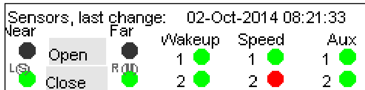
Sensor status window from RailBAM® web page and GUI, showing 'Speed Sensor 2' engaged
