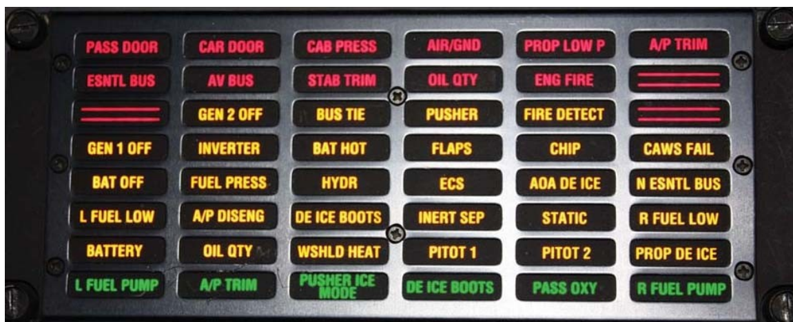
Figure 5. Central advisory and warning system display.
