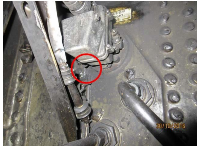
PHOTO 45: RIGHT ENGINE FUEL SHUTOFF VALVE IN CLOSED POSITION
