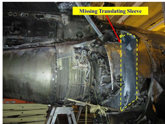
PHOTO 24: OUTBOARD TRANSCOWL SLEEVE DAMAGE
