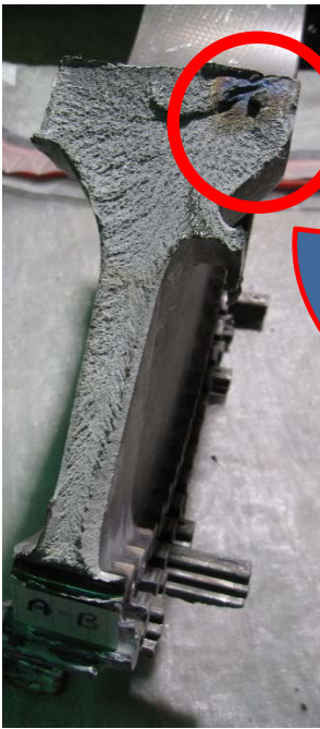
PHOTO 48: HPT STAGE 2 DISK FRACTURE SURFACE FOR FRAGMENT 'A' THAT MATCHES WITH FRAGMENT 'B'
