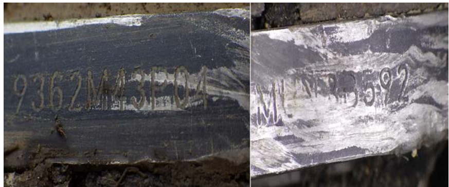
PHOTO 2: PART MARKING ON THE HPT STAGE 2 DISK LOCATED ON TOP OF DISK POST FRAGMENT ‘B’ – PN ON LEFT AND SN ON RIGHT
