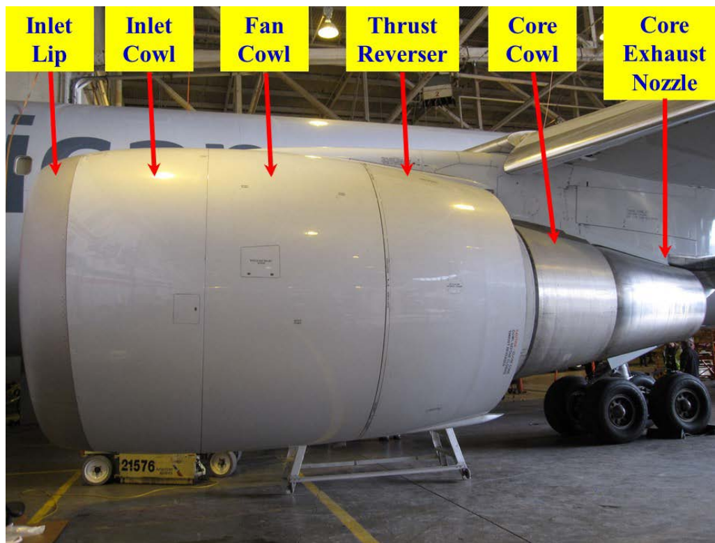
PHOTO 3: BOEING 767-300/GE CF6-80C2 INSTALLATION NACELLE NOMENCLATURE AND LOCATION PICTURE IS OF THE SISTER ENGINE (LEFT) ON THE EVENT AIRPLANE
