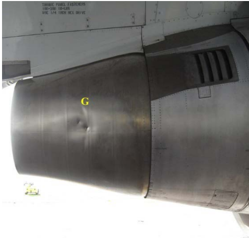
PHOTO 6: EXHAUST NOZZLE DAMAGE
