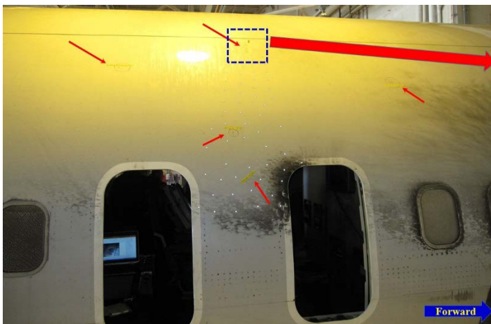
PHOTO 38: DEBRIS IMPACT MARK ON RIGHT SIDE OF FUSELAGE NEAR THE OVERWING DOORS
