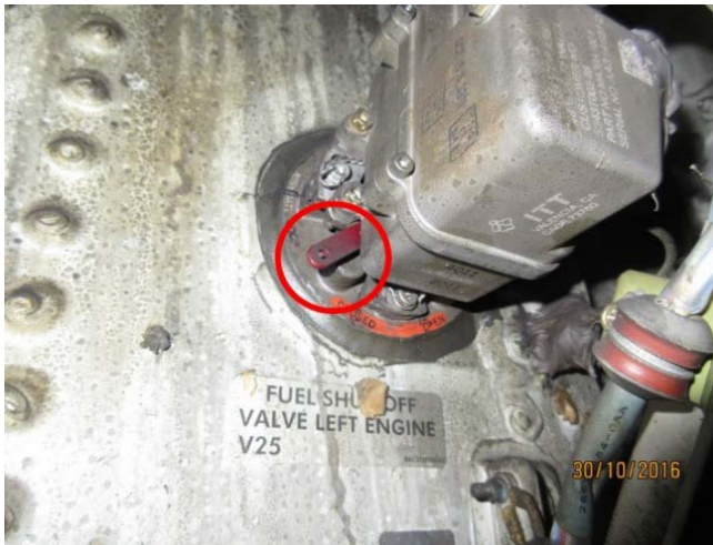
PHOTO 44: LEFT ENGINE FUEL SHUTOFF VALVE IN CLOSED POSITION
