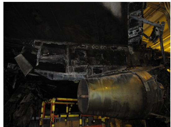
PHOTO 29: OUTBOARD PYLON/STRUT DAMAGE
