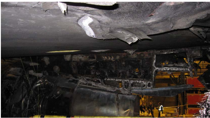
PHOTO 28: INBOARD PYLON/STRUT THERMAL DAMAGE
