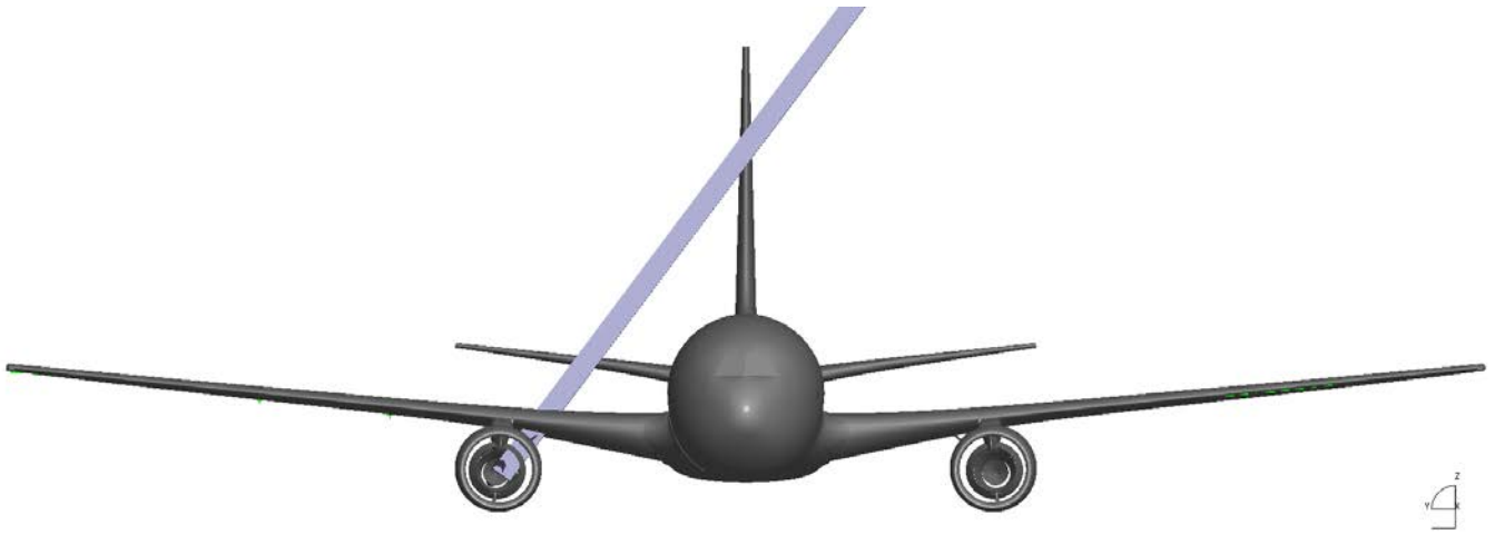
FIGURE 27: HPT STAGE 2 DISK FRAGMENT EXIT TRAJECTORY THROUGH INBOARD RIGHT WING (FORWARD LOOKING AFT)
