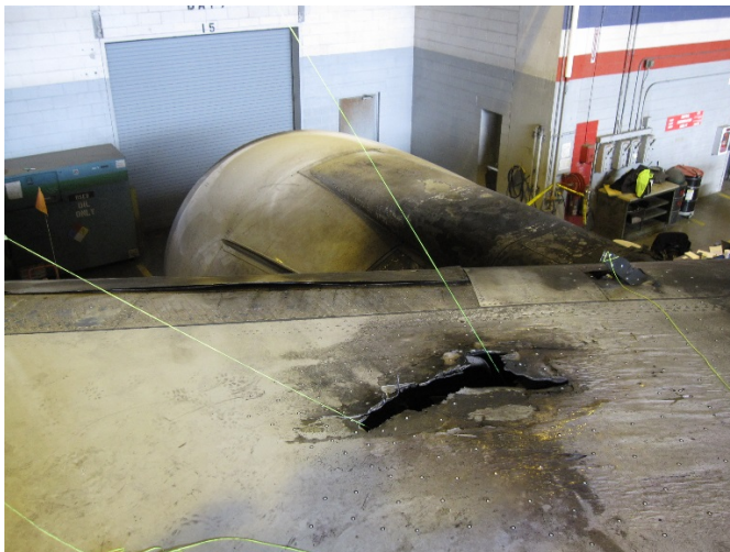
PHOTO 32: RIGHT WING INBOARD OF PYLON UPPER WING SKIN THRU-HOLE PENETRATION – HOLE ②
