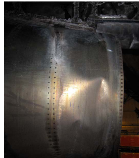
PHOTO 27: BUCKLED CORE EXHAUST NOZZLE
