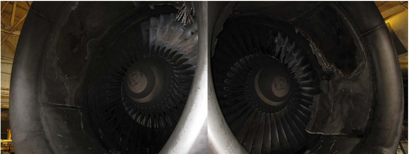
PHOTO 20: INLET COWL DAMAGE – MISSING ACOUSTIC LINER AND DAMAGED HONEYCOMB
