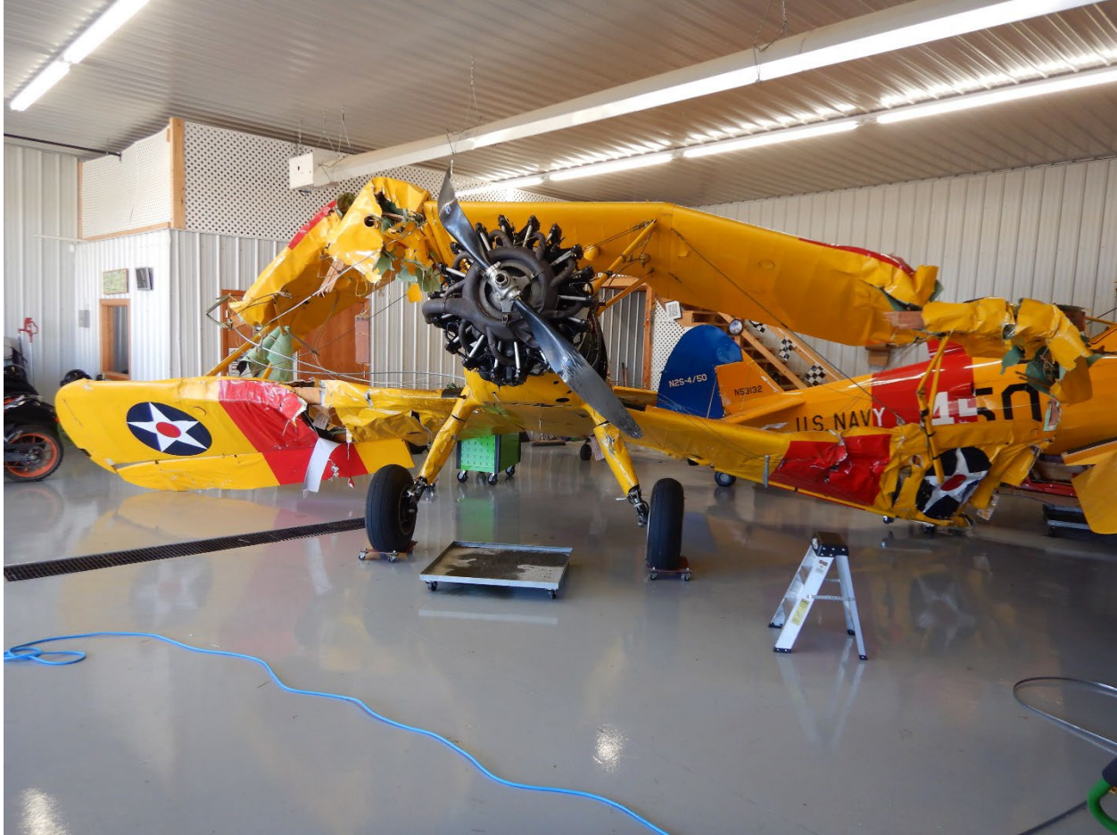
Figure 4. Upper and lower wings, showing substantial damage.
