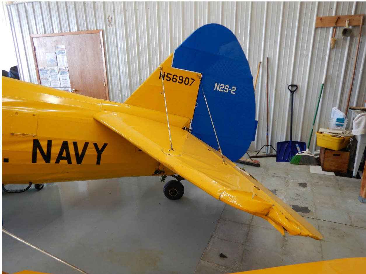
Figure 3. Empennage, left side, showing substantial damage to the horizontal stabilizer.
