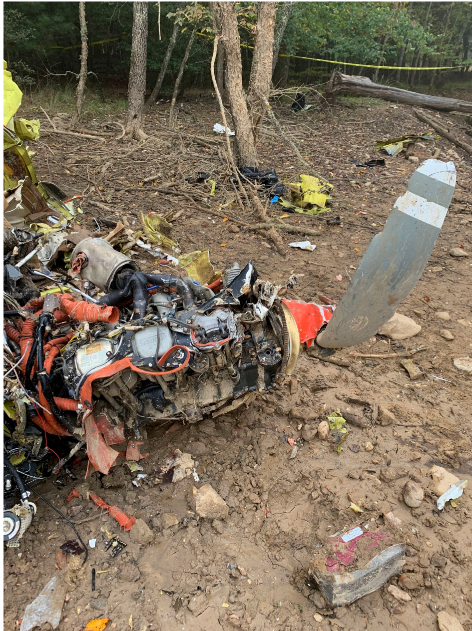
Photo 6 – Engine and Propeller (NTSB Photo)
