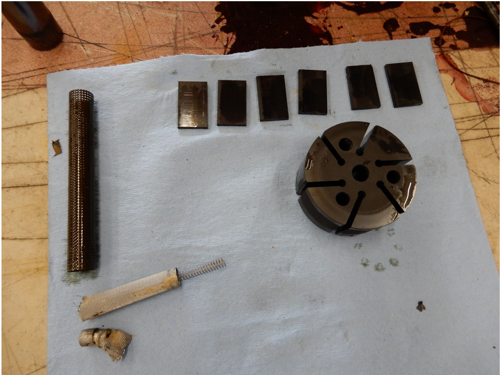
Photo 9 – Vacuum Pump Rotor and Vanes (NTSB Photo)
