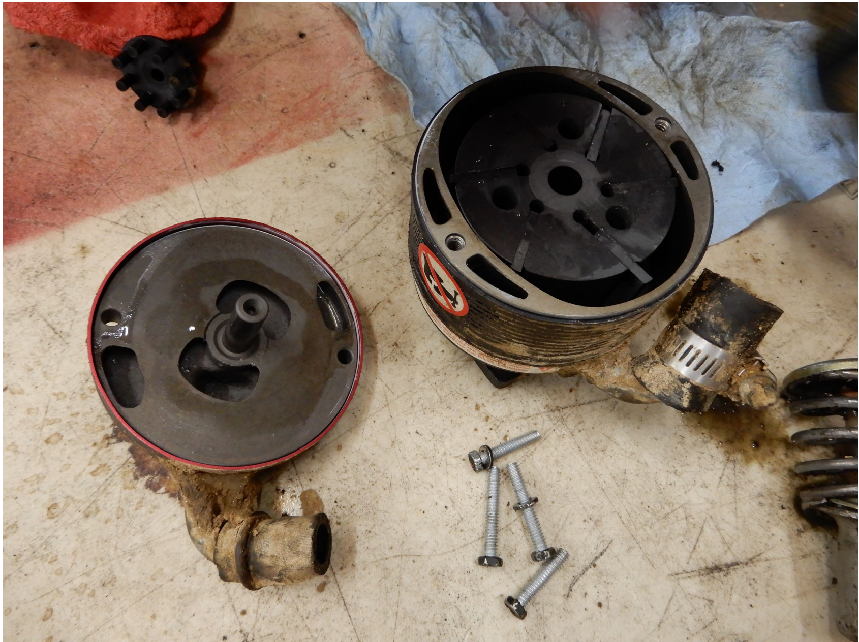
Photo 8 – Engine-driven Vacuum Pump (NTSB Photo)
