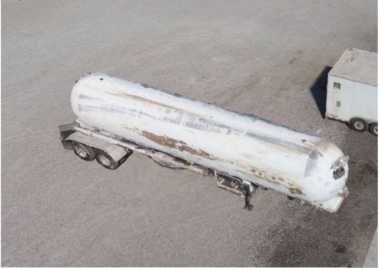
Figure 5. Image of the generated three-dimensional point cloud of the involved tanker trailer.
