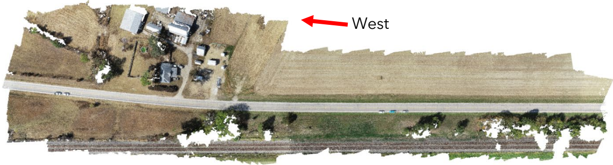
Figure 2. Image of the generated point cloud of the crash scene.
