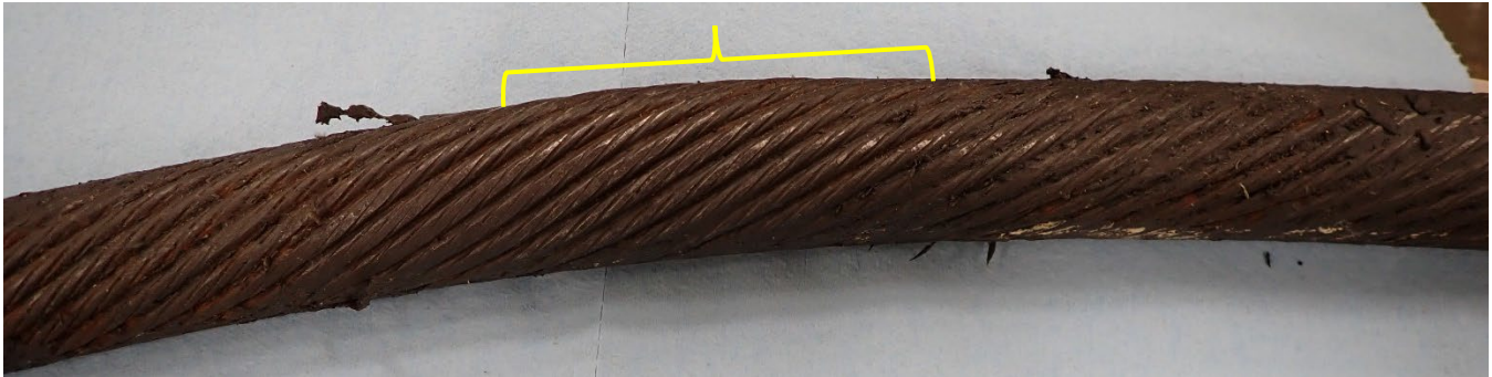
Figure 12 Image showing the local increase in rope diameter observed at the 48-inch mark on Specimen 1 (74-1, the eye piece).
