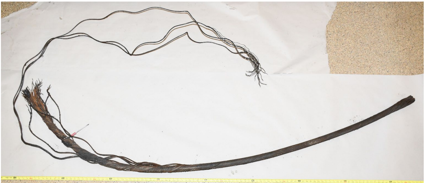
Figure 2 Images showing Specimen 2 (76, the crane-side of the fracture).
