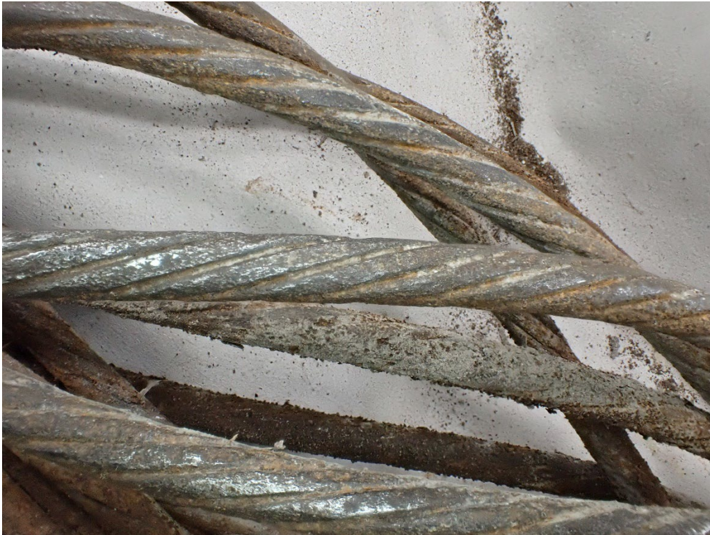
Figure 9 Representative image showing the rough surface or pitting observed on Specimen 3 (78-1, block-side of fracture). (79-inches from reference end, Severity Rating 60%)
