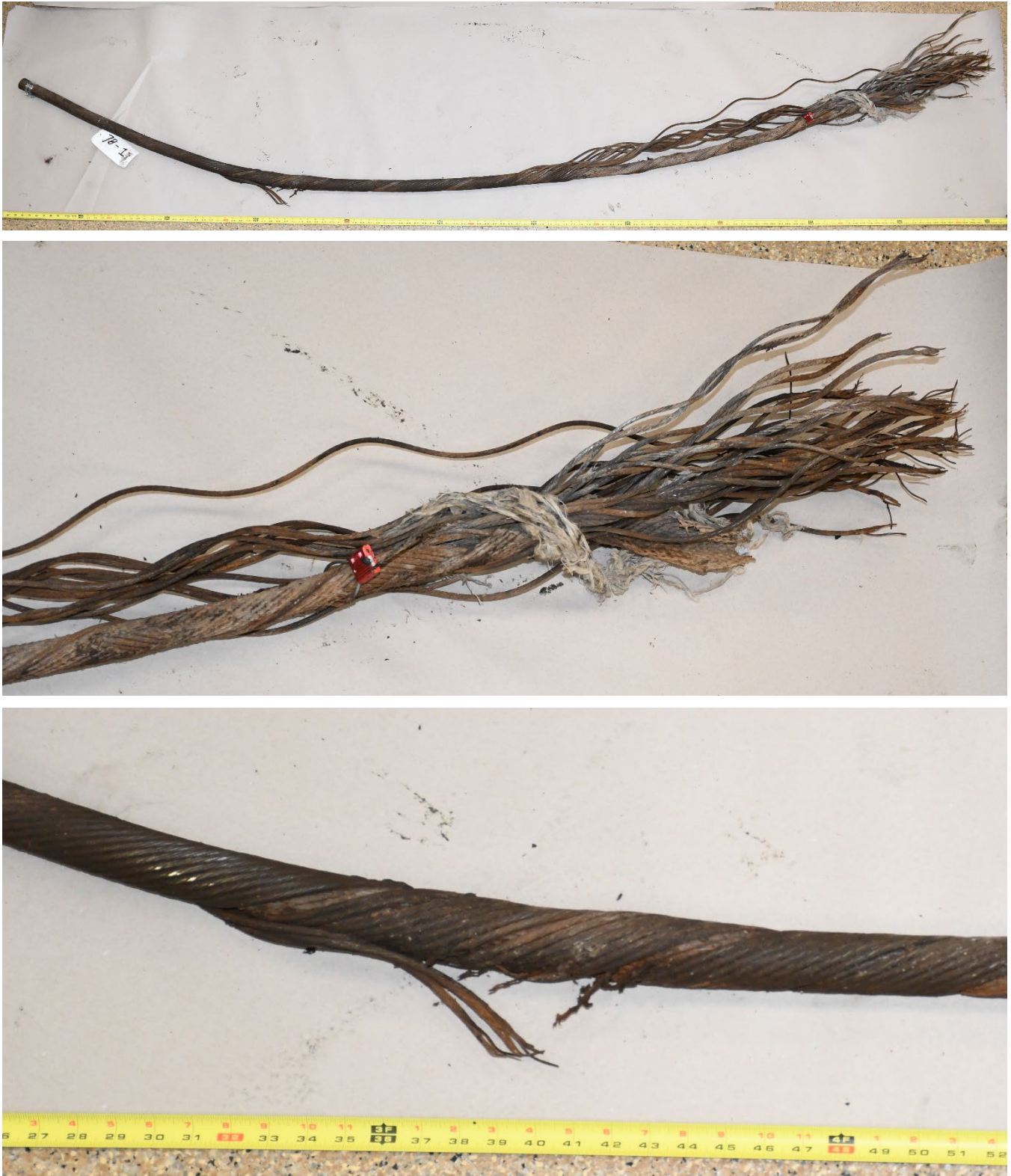
Figure 3 Images showing Specimen 3 (78-1, the block-side of the fracture) after sectioning 10 feet from the fractured end.
