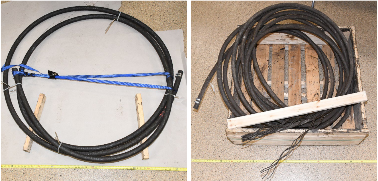
Figure 4 Images showing the excess lengths of wire rope from Specimen 1 (74-2, the eye piece, lefthand image) and Specimen 3 (78-2, the block-side of the fracture, righthand image) after removal of 10-foot sections.
