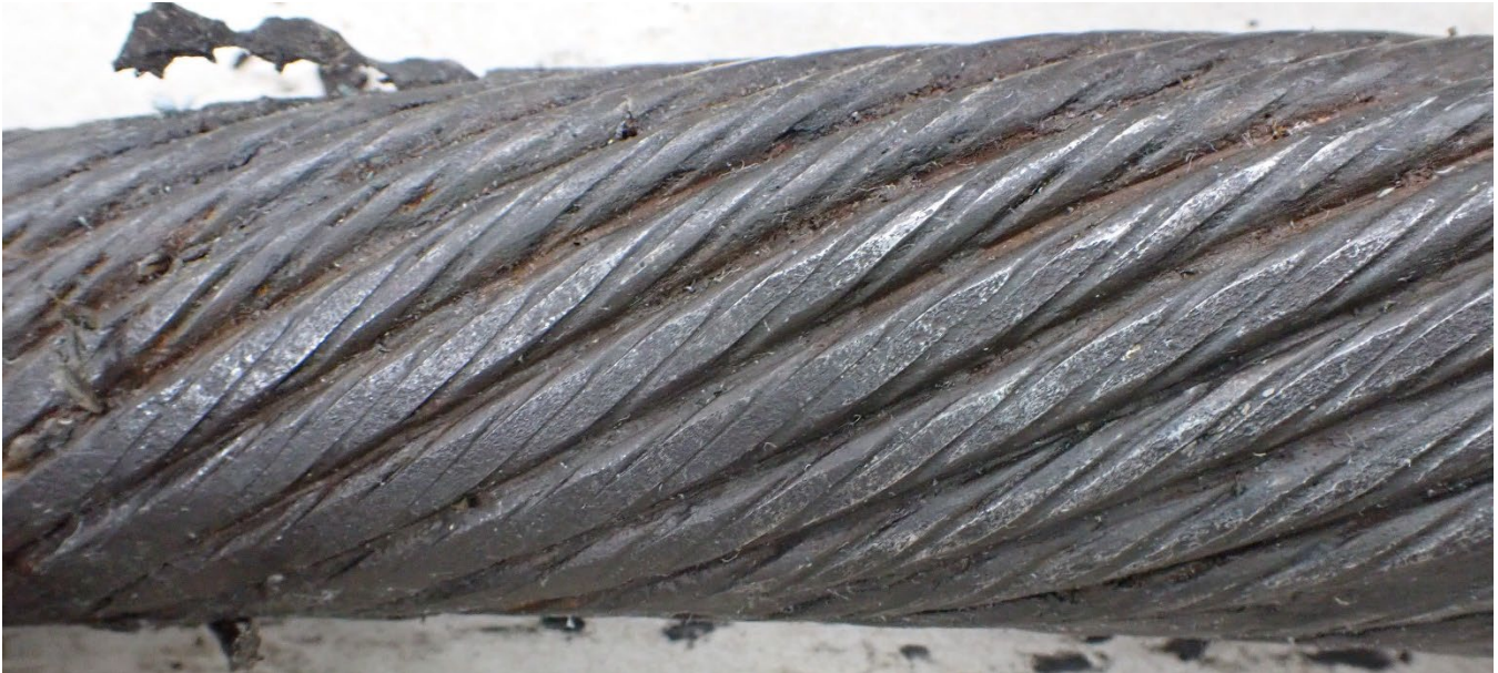
Figure 10 Representative image showing the external wear observed at the 48-inch mark on Specimen 1 (74-1, the eye piece).
