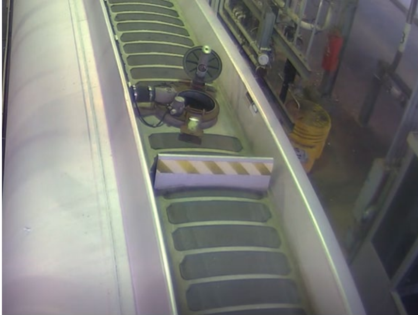
Figure 3 - Open Manhole Compartment #1 (Source: Buckeye Terminal)
