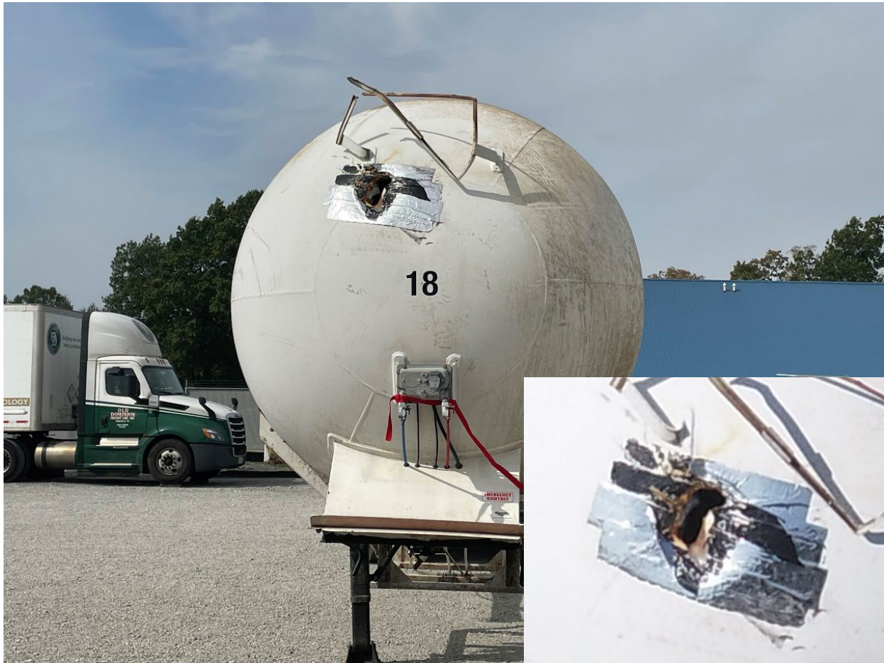
Figure 9. Image of the cargo tank semitrailer head depicting puncture.
