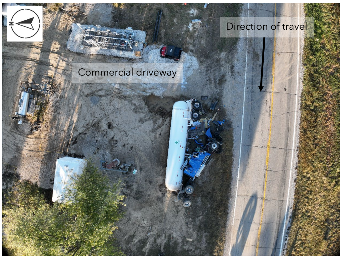
Figure 6. Overhead image of the combination vehicle at final rest. (Source: ISP edited by NTSB)
