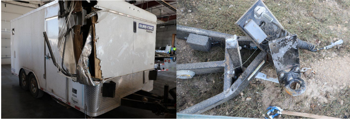
Figure 10. Photograph depicting the damage to the right front corner of the trailer. Right photograph shows damage to the tongue and lunette ring (Source: ISP).
