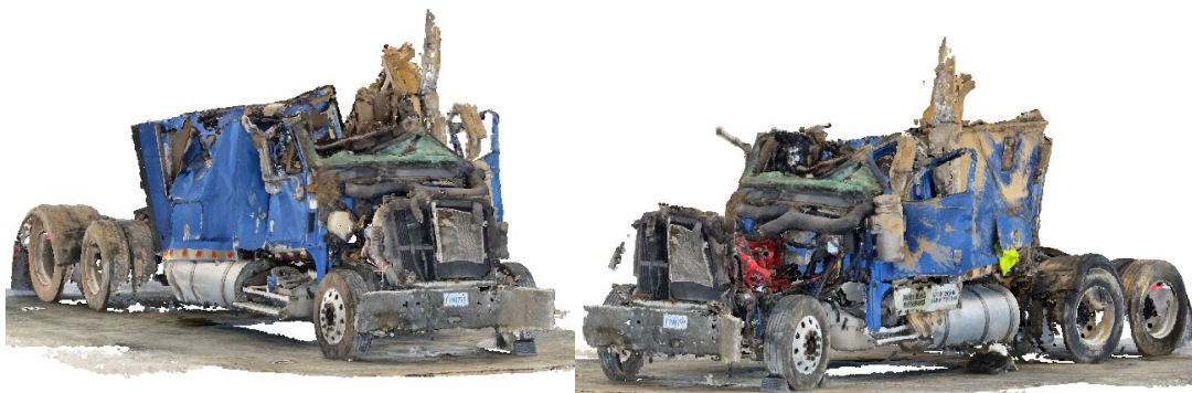
Figure 7. Three-dimensional point cloud images of the of the International truck tractor depicting the damage sustained from the crash.
