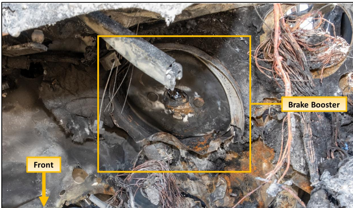
Figure 13. Rear plate of the brake booster.
