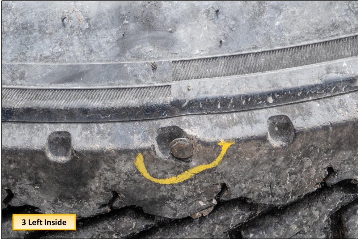
Figure 23. Object stuck in the tread of the left inside tire on axle 3.
