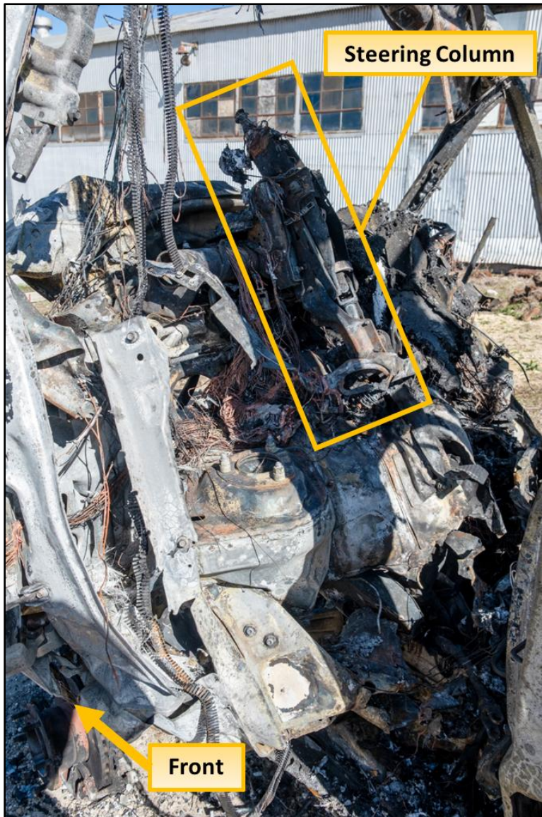
Figure 4. The condition of driver controls at inspection of the Micro Bird.
