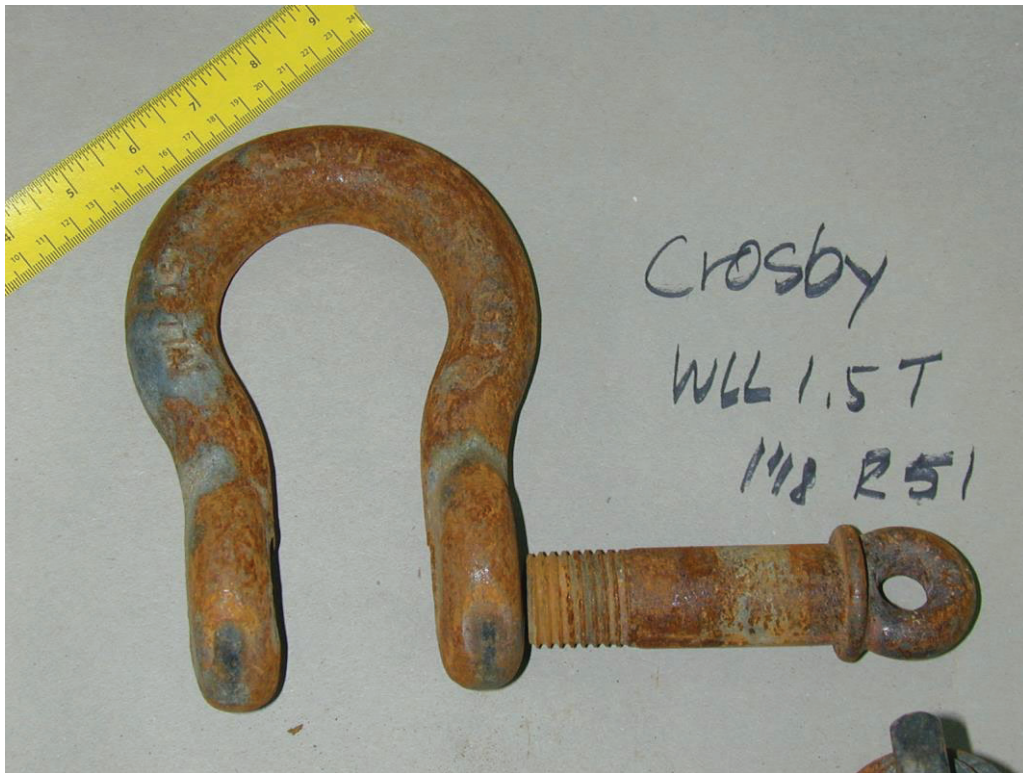
Fig. 7: Close up view of the Crosby shackle.
