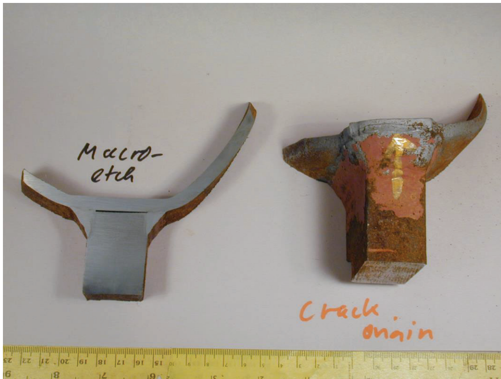
Fig. 26: Close up view of the macro-etched weld x-section and ultrasonically cleaned failure origin.
