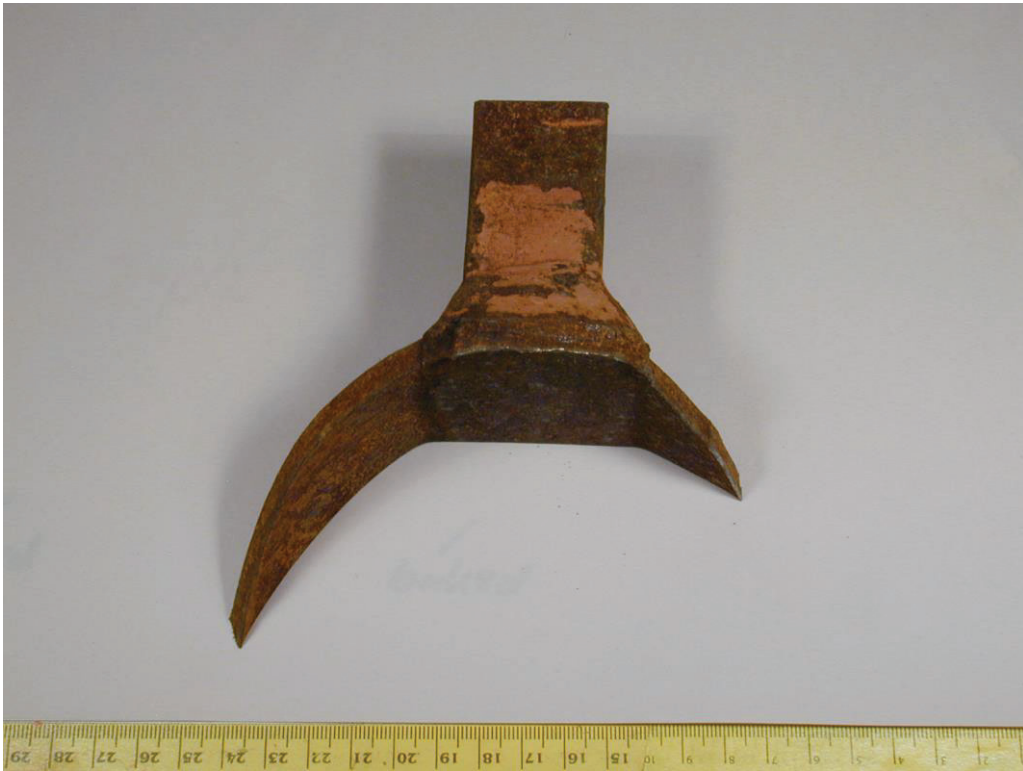
Fig. 19: Overall view of the liberated failure origin.
