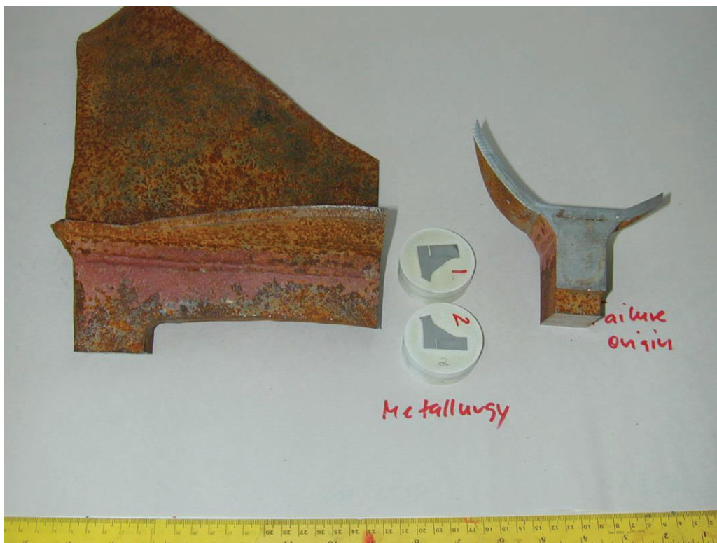
Fig. 40: Same as Fig. 39, but the cleaned failure origin is shown from the end.
