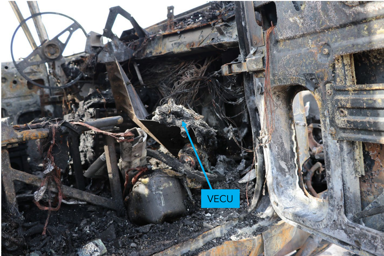
Figure 12. Photograph showing the VECU.
