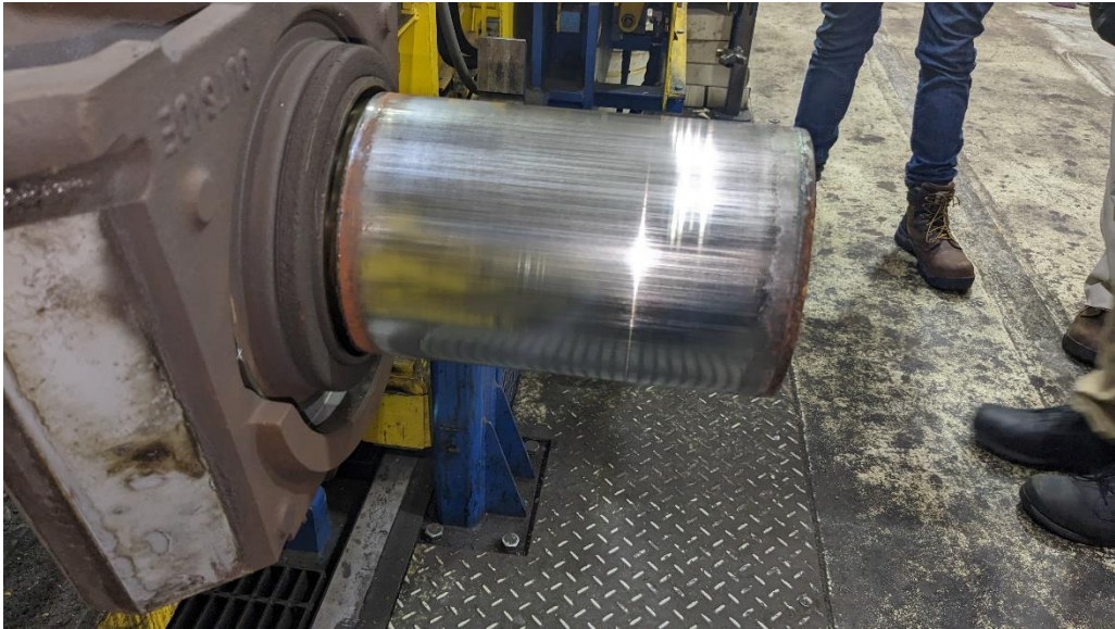
Figure 23: Motor Side Wheelseat
