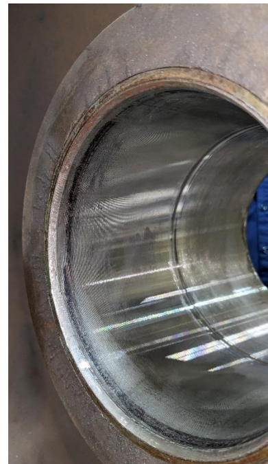
Figure 17: Motor Side Wheel Bore Cleaned
