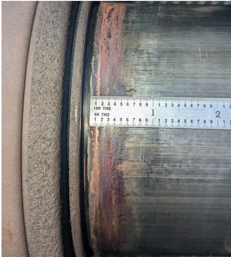
Figure 22: Gear Side Wheel Fretting with Scale
