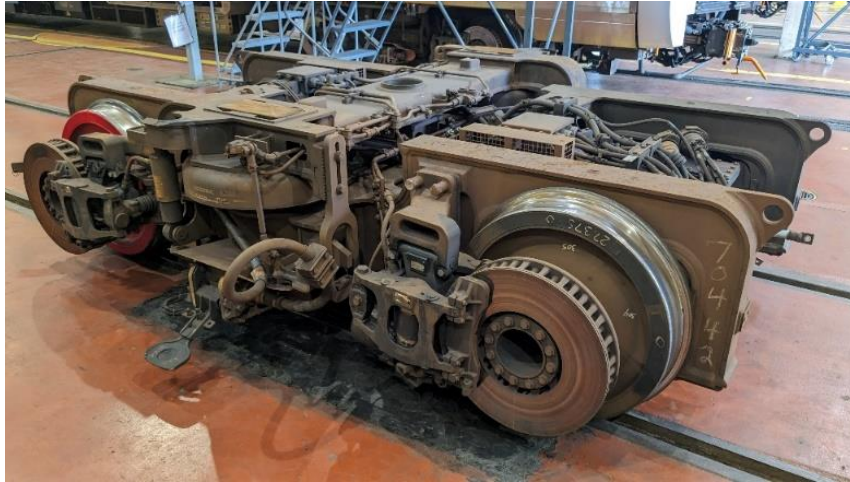
Figure 5: Removed Front Truck SN 70442
