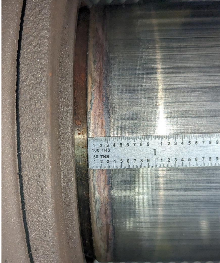
Figure 26: Motor Side Wheelseat Fretting with Scale
