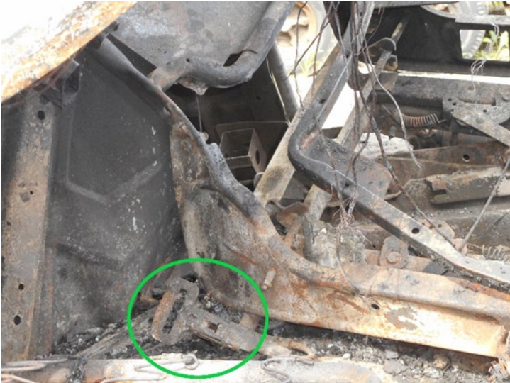
Figure 6. View of truck driver's seat belt latchplate still buckled (circled in green).
