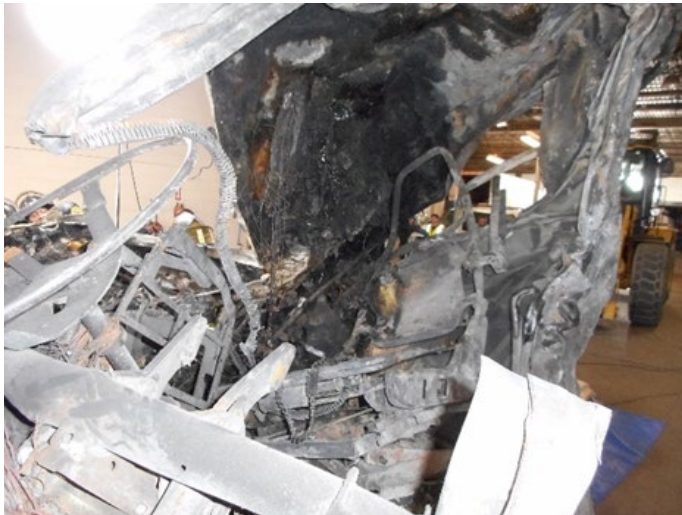
Figure 4. Interior view of cab deformation and intrusion.
