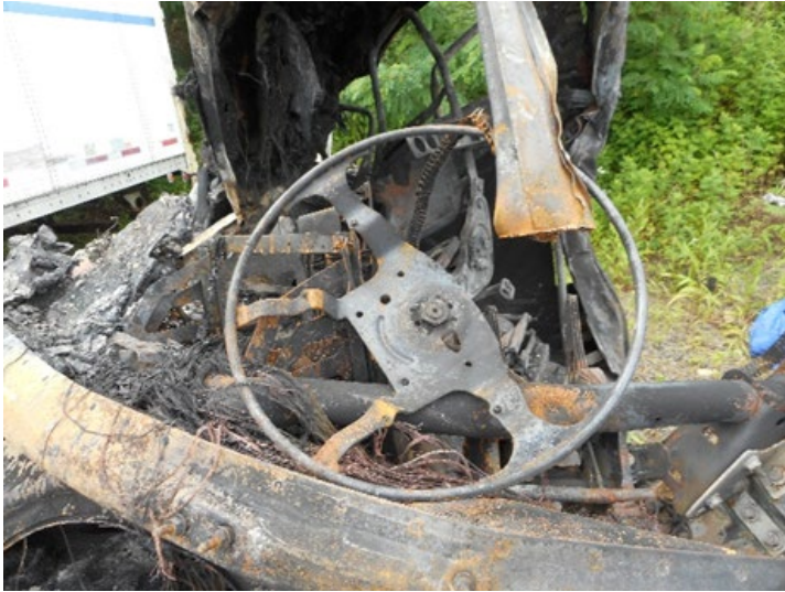
Figure 5. View of undeformed steering wheel.
