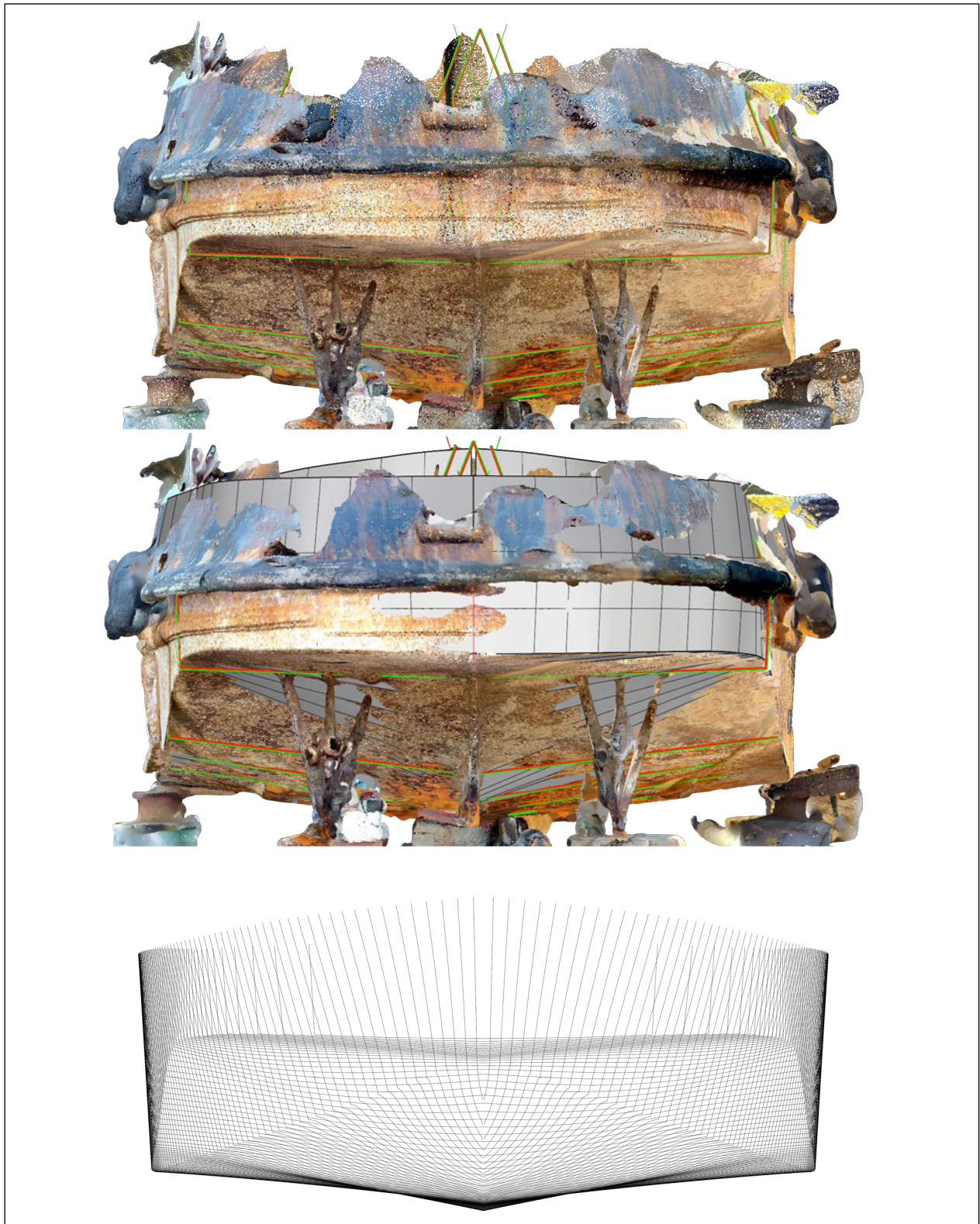
Figure 3: Modeling Progression: Point Cloud and Offsets (top), Surfaces Fit Through Point Cloud and Offsets (middle), Lines Plan (bottom)
