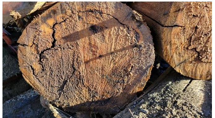
203. Degraded core of top section
