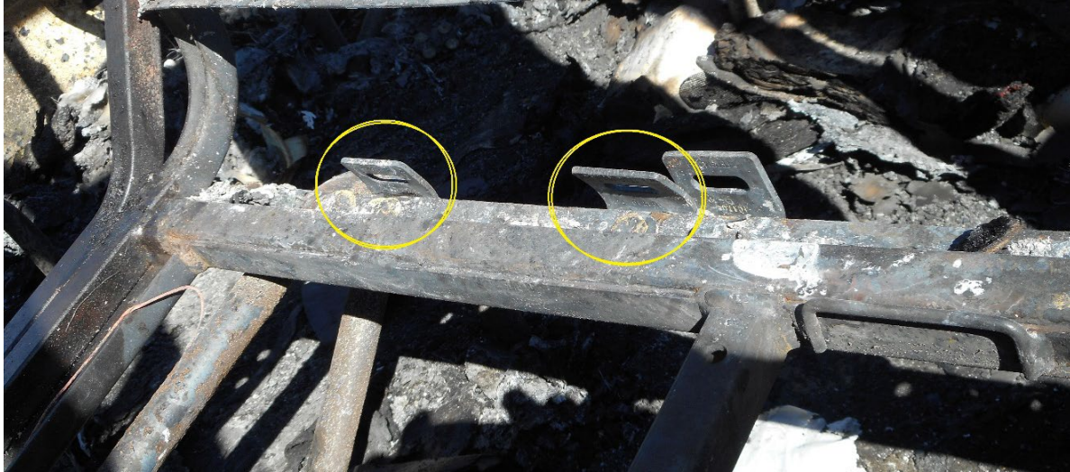
Figure 6. View of bent lap belt anchors (circled) on the seat frame in Row 1 left side aisle seat.
