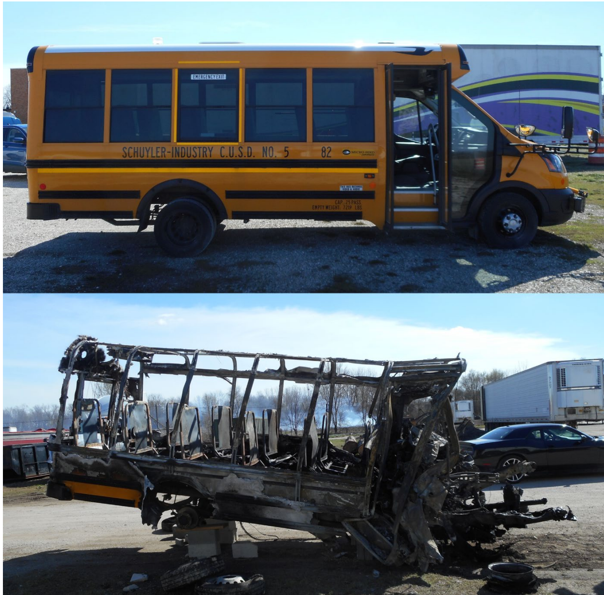
Figure 3. Comparison view of right side of exemplar bus and damage to crash bus.
