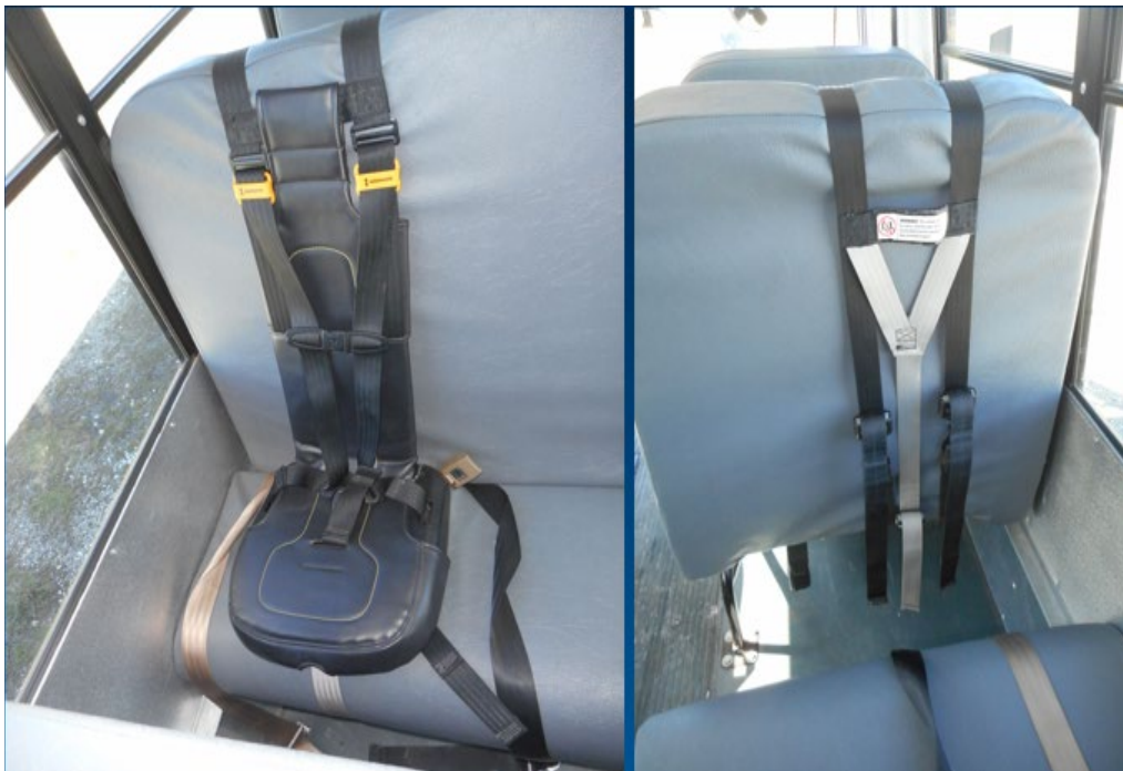
Figure 7. Front and rear views of installed 5-point CSRS in exemplar school bus.
