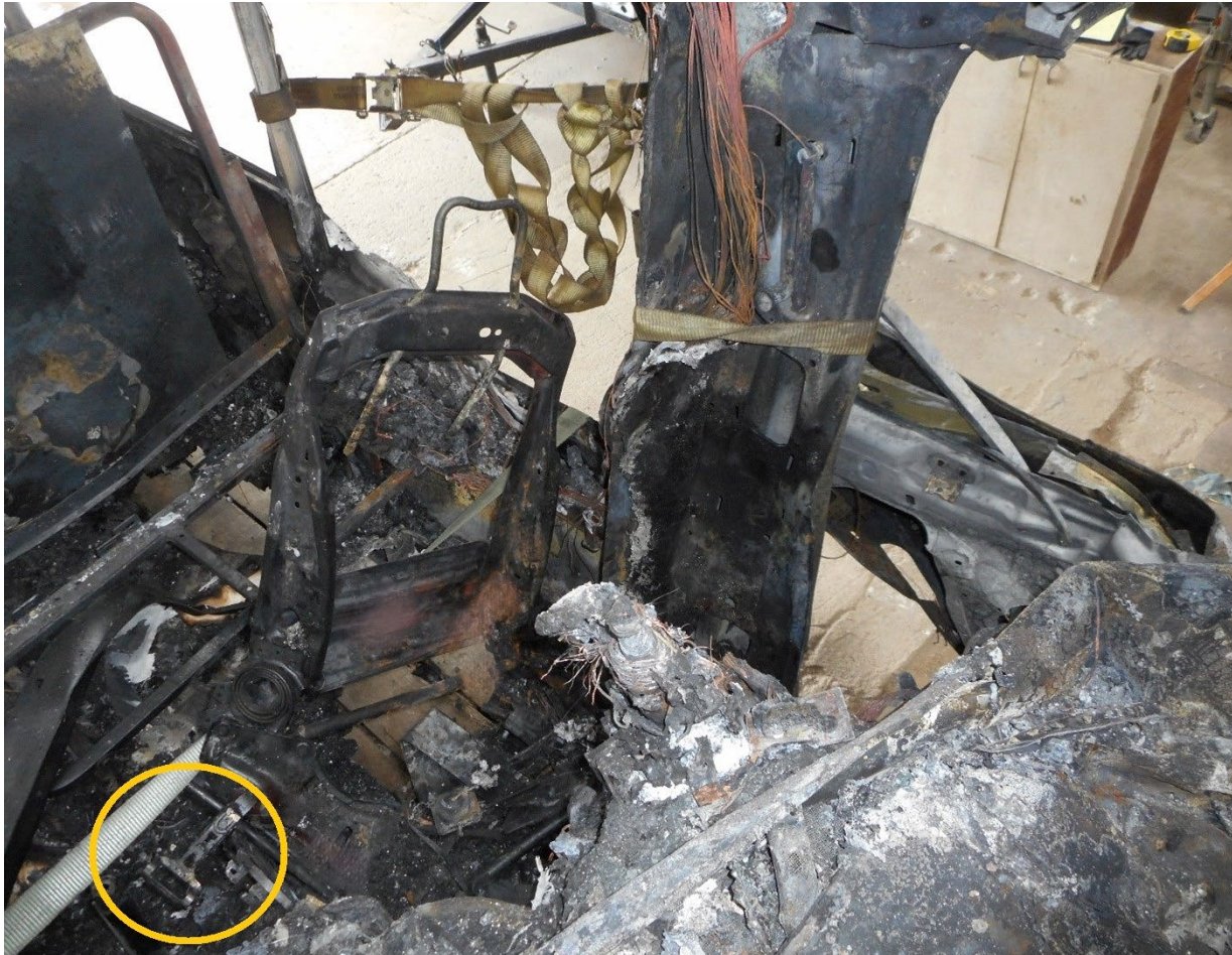
Figure 5. Overhead view of deformation to driver's seating area. Note buckled seatbelt (circled).
