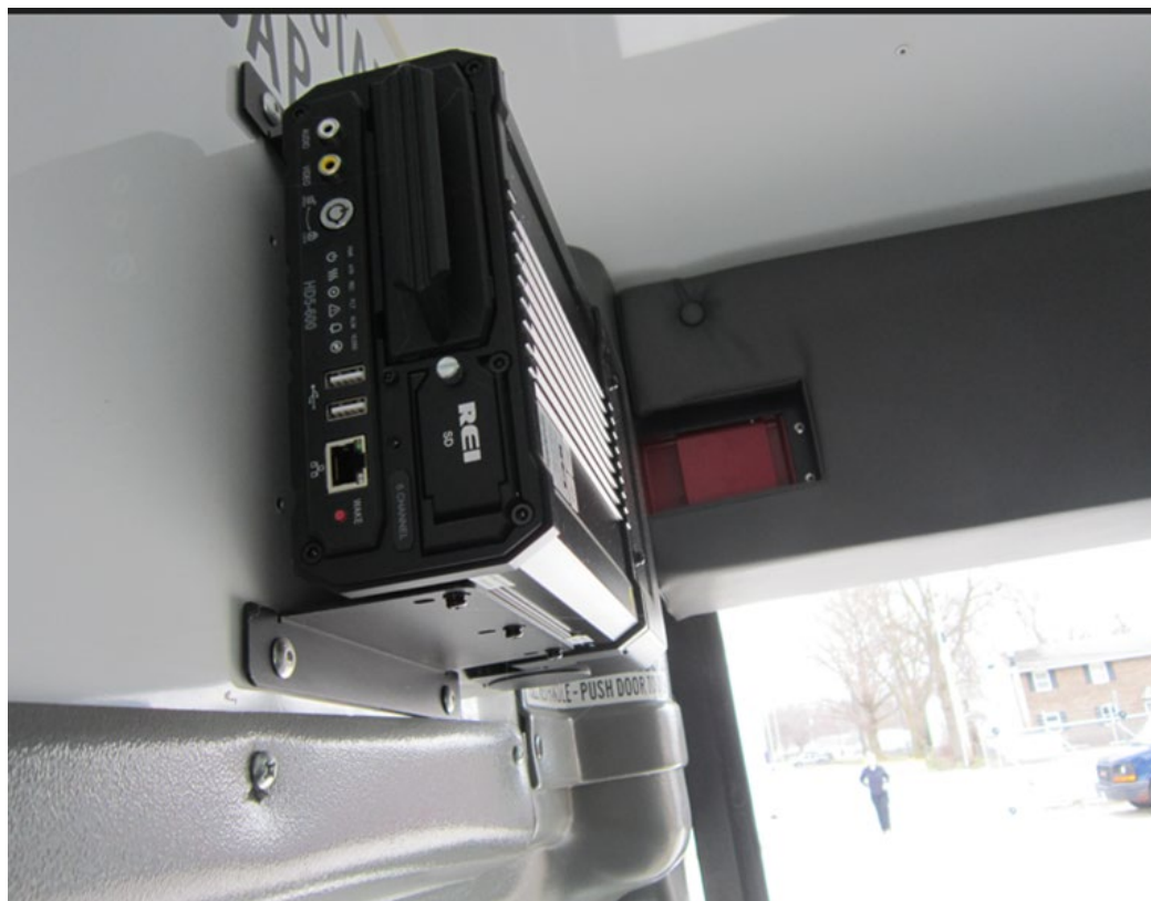
Figure 12. REI hard drive recording system in exemplar school district school bus.
