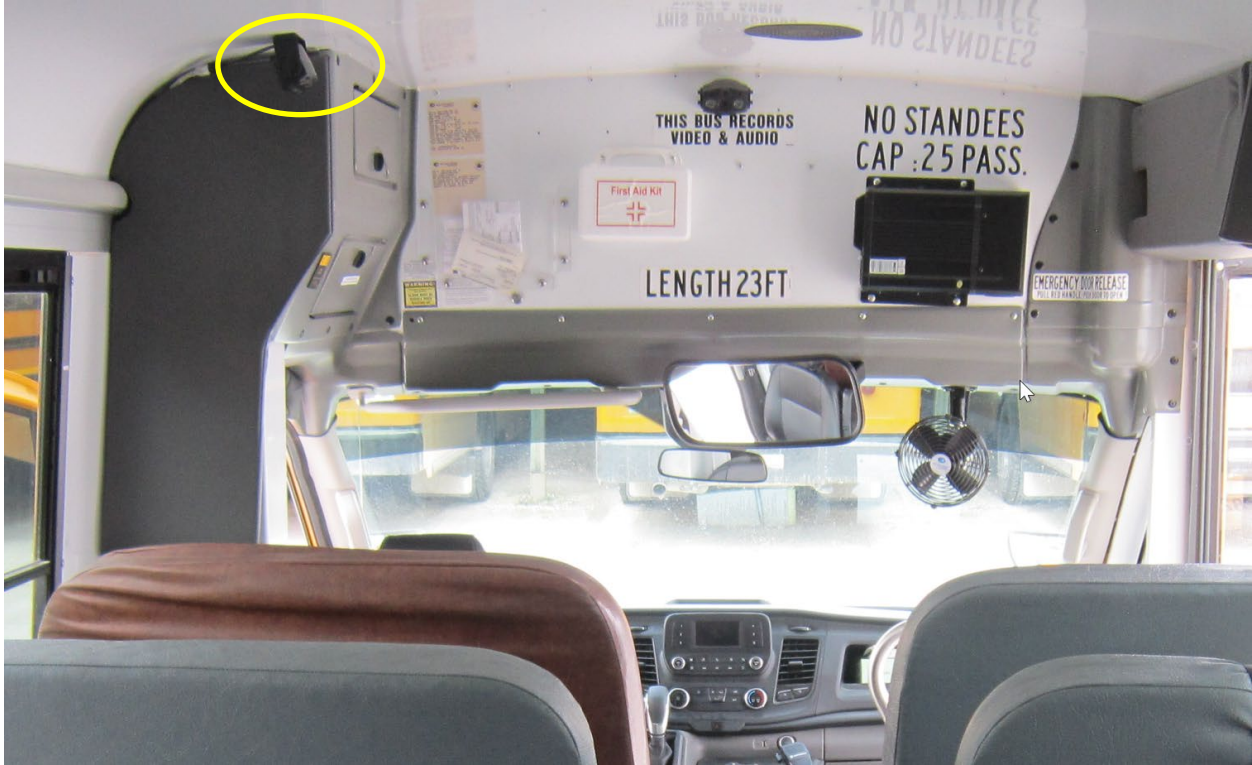
Figure 10. Camera mounted left side of driver (highlighted in the yellow oval).
