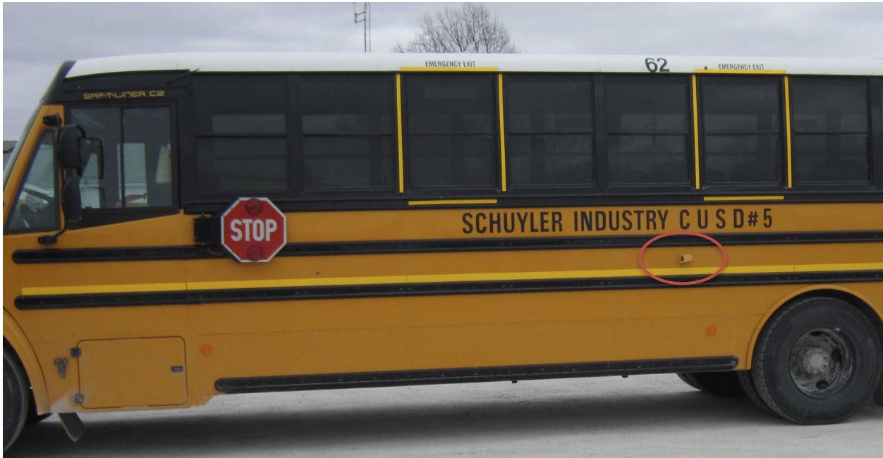
Figure 11. External camera for stop arm violators (highlighted in red oval).
