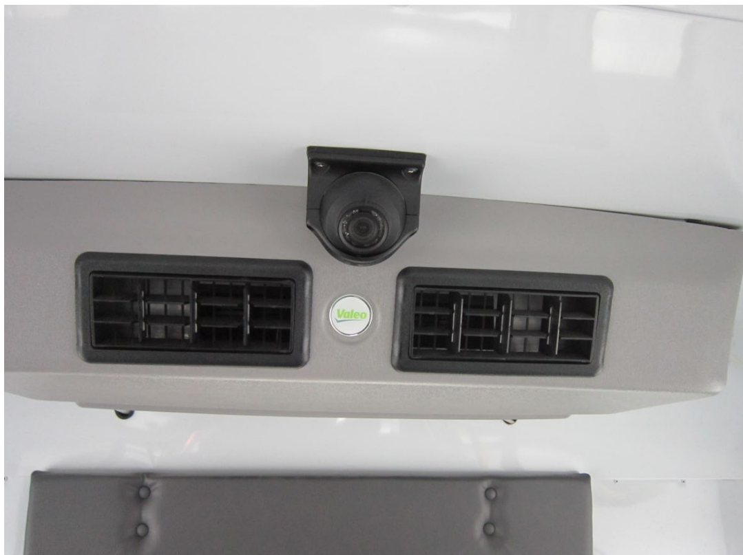
Figure 9. Forward facing video camera mounted at rear of bus.
