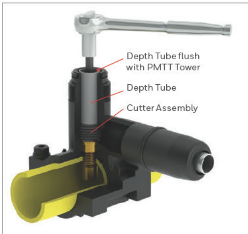
Fig. 4 - Full installation of Cutter Assembly, Cutter Sleeve engaged in (PE) Main, Depth Tube is flush with top of PMTT Tower
