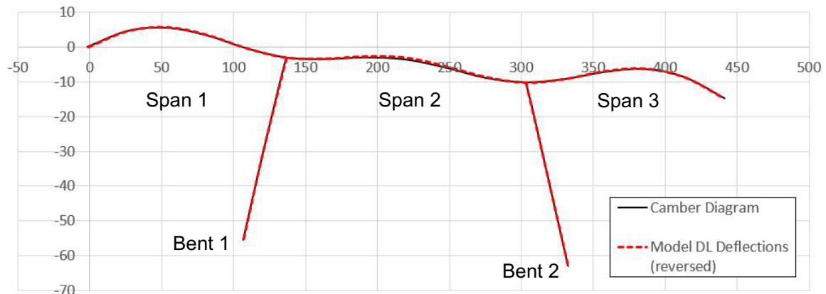
Figure 5 – Plot of cambered shape in drawings vs. reversed dead load deflections in analysis mode (longitudinal positions in feet, deformations in feet amplified 30x).
