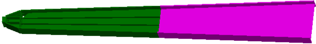
Figure 7 – Local FEA model of frame leg
