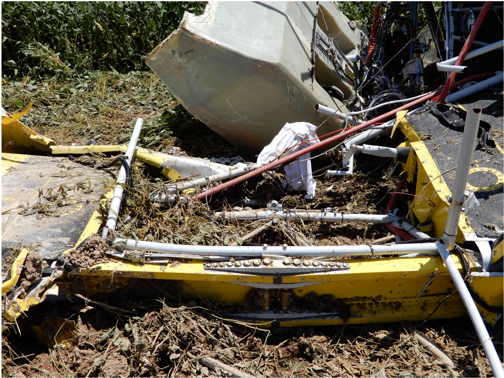
Photo 13 - N749LA Main Spar Carry-Through (NTSB Photo)
