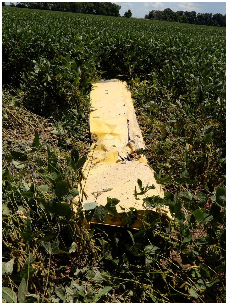
Photo 15 - N749LA Right Wing Flap (NTSB Photo)
