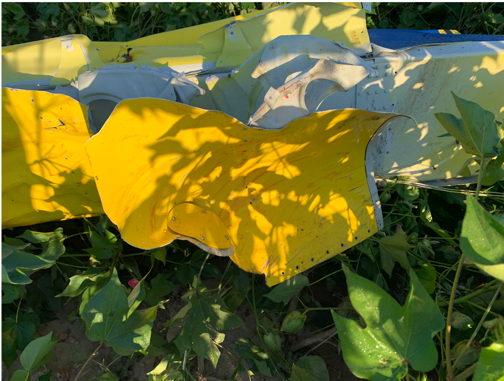
Photo 5 - N214RL Left Wing Damage (NTSB Photo)
