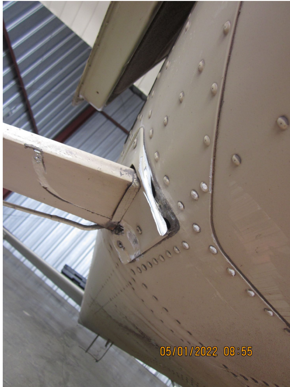
Photo 5 – Landing Gear Strut Attachment (FAA Photo)
