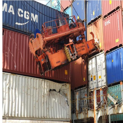
CGM CMA BIANCA Container Spreader impaled into cargo container following wind event.
