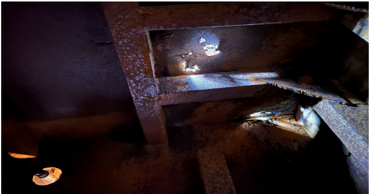
Hole #3 and stern hole viewed from inside lazarette after bulwark steel cropped out. Hole possibly enlarged by scale removal.
