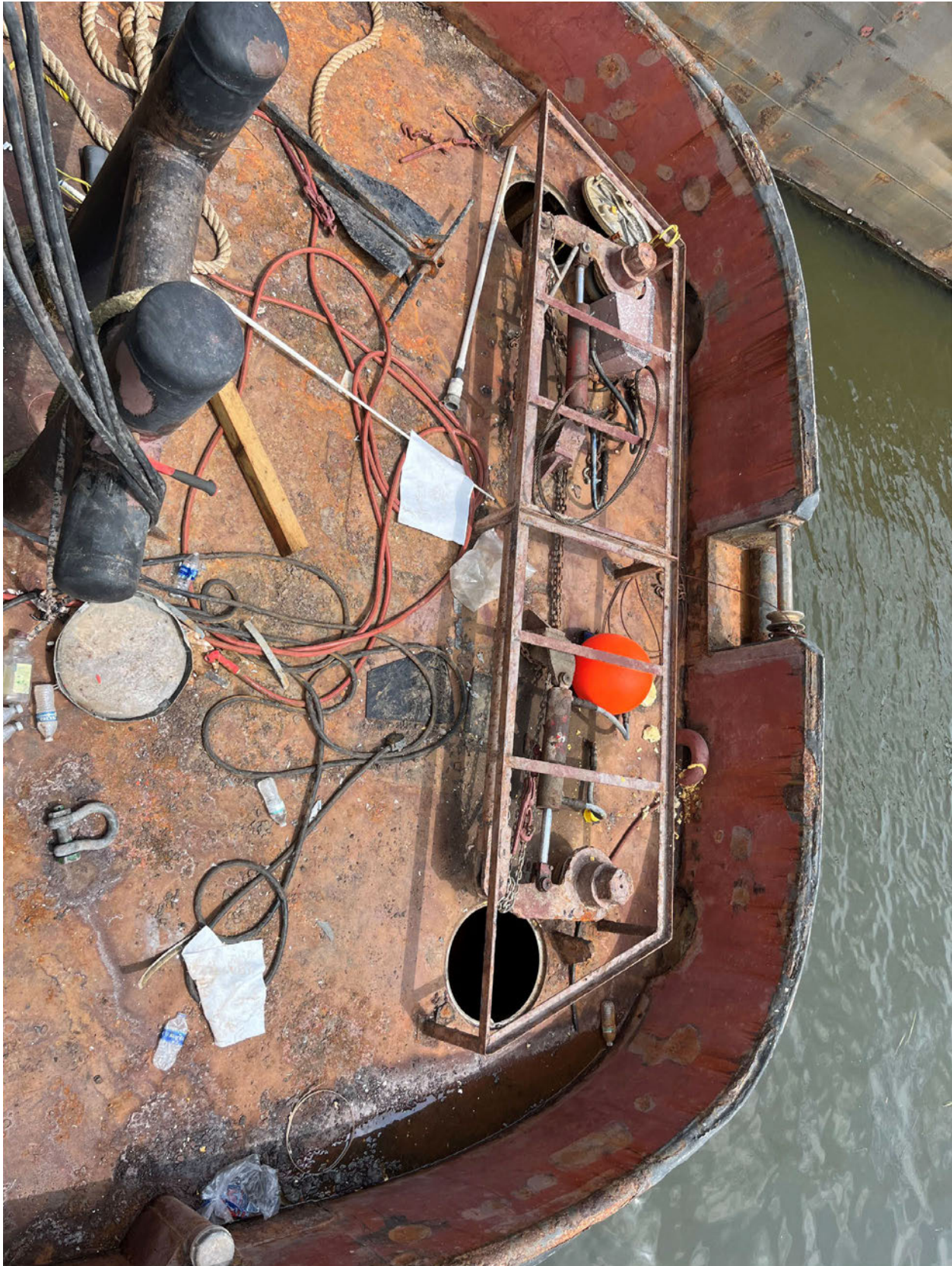
Inboard view of closed bulwark prior to steel being cropped out.
