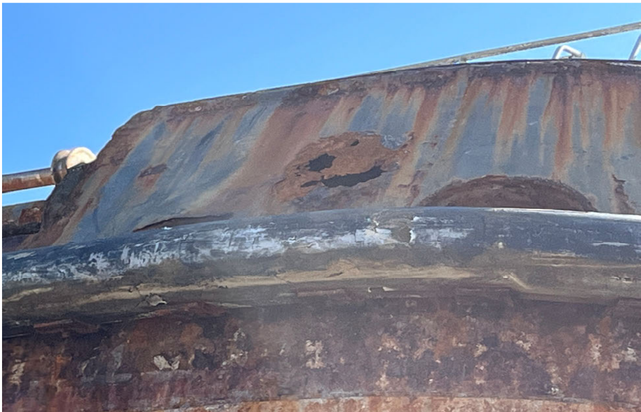
Stern view of closed bulwark with plate wastage.
