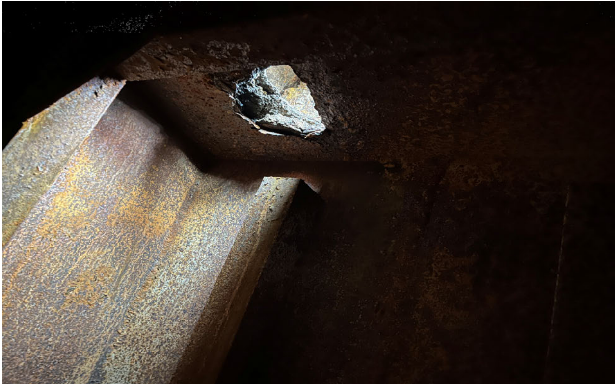
Hole #1 viewed from inside lazarette after bulwark steel cropped out. Hole possibly enlarged by scale removal.
