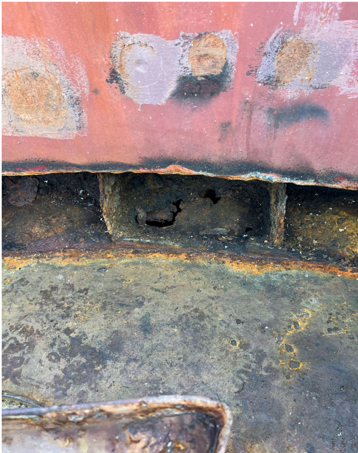
Hole #2 in way of frame #'s 2 and 3 after bulwark steel cropped out. Hole possibly enlarged by scale removal.
