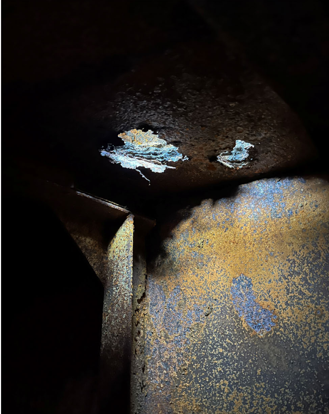
Hole #2 viewed from inside lazarette after bulwark steel cropped out. Hole possibly enlarged by scale removal.
