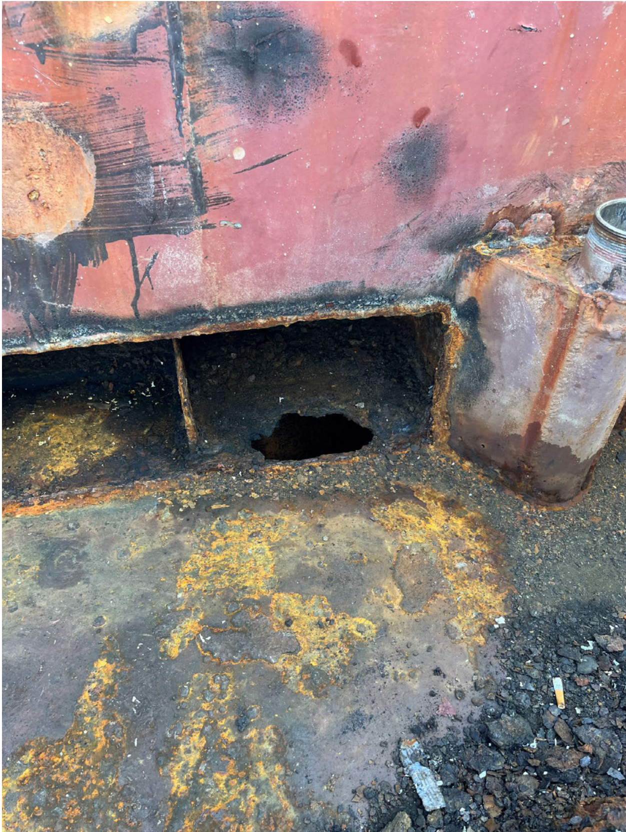
Hole #1 port side adjacent to lazarette forward bulkhead after bulwark steel cropped out. Hole possibly enlarged by scale removal.
