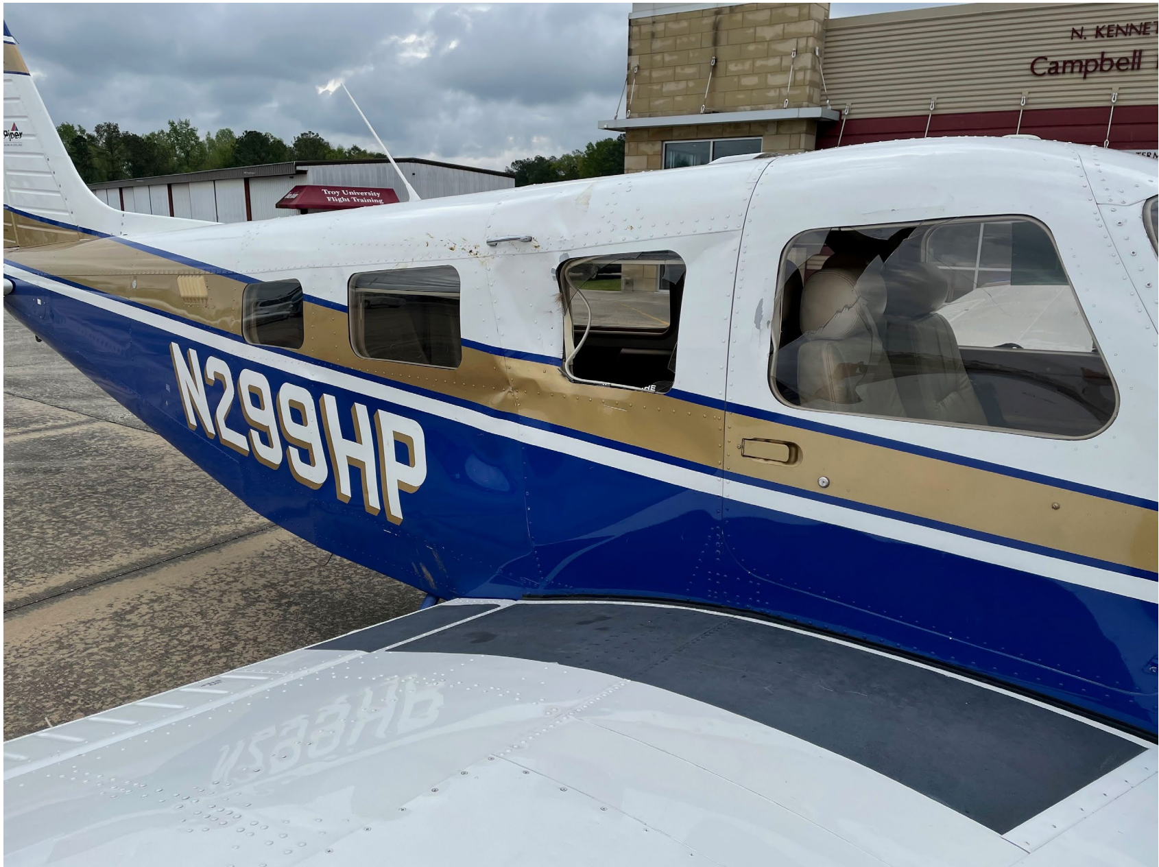
Photo 1 – N299HP Fuselage Damage (FAA Photo)
