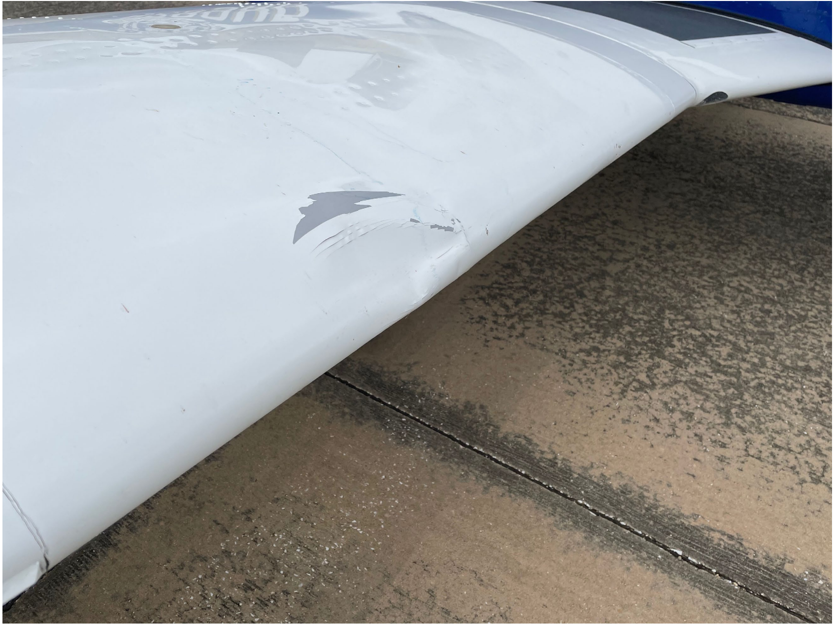
Photo 4 - N299HP Right Wing Damage (FAA Photo)
