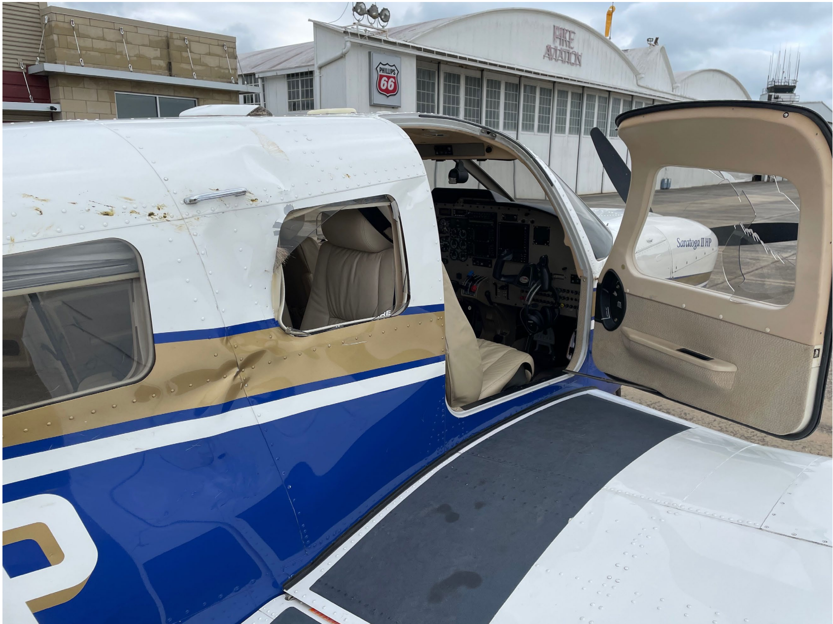
Photo 2 – N299HP Fuselage Damage (FAA Photo)
