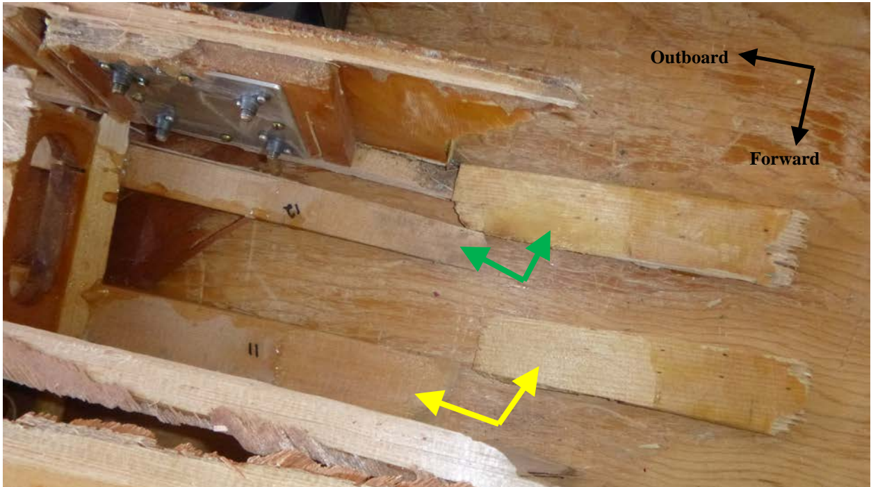
Figure 4 – Forward spar lower spar cap fractures
