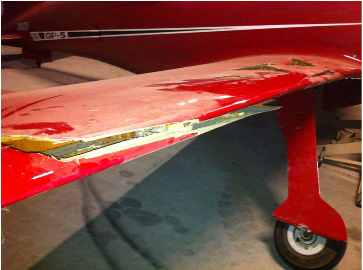
Figure 6 – Right wing upper surface damage following March 11, 2012, landing
