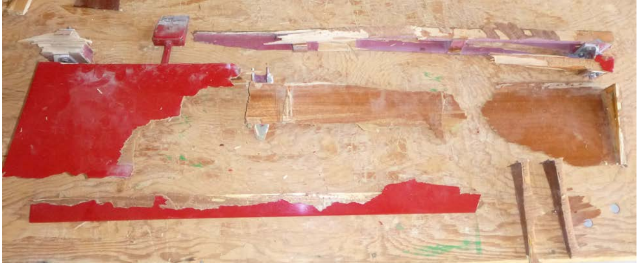
Figure 5 – GP-5 right aileron reconstruction
