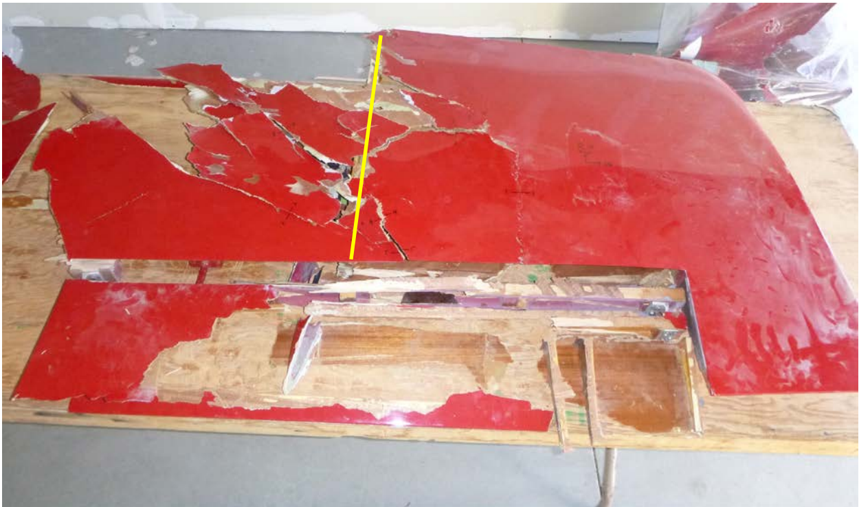
Figure 2 – GP-5 right wing reconstruction, upper surface
