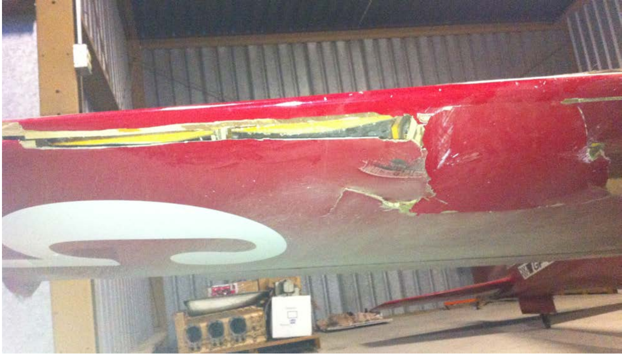
Figure 7 – Right wing lower surface damage following March 11, 2012, landing
