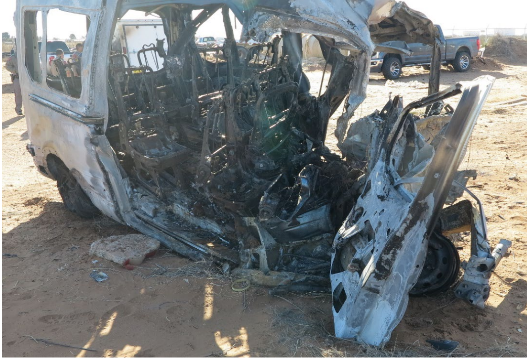
Photograph 5: A view of the damage sustained at the right front of the van
