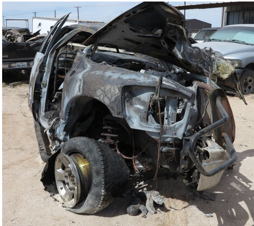
Photograph 2: A view of the damage sustained at the right front of the pickup
