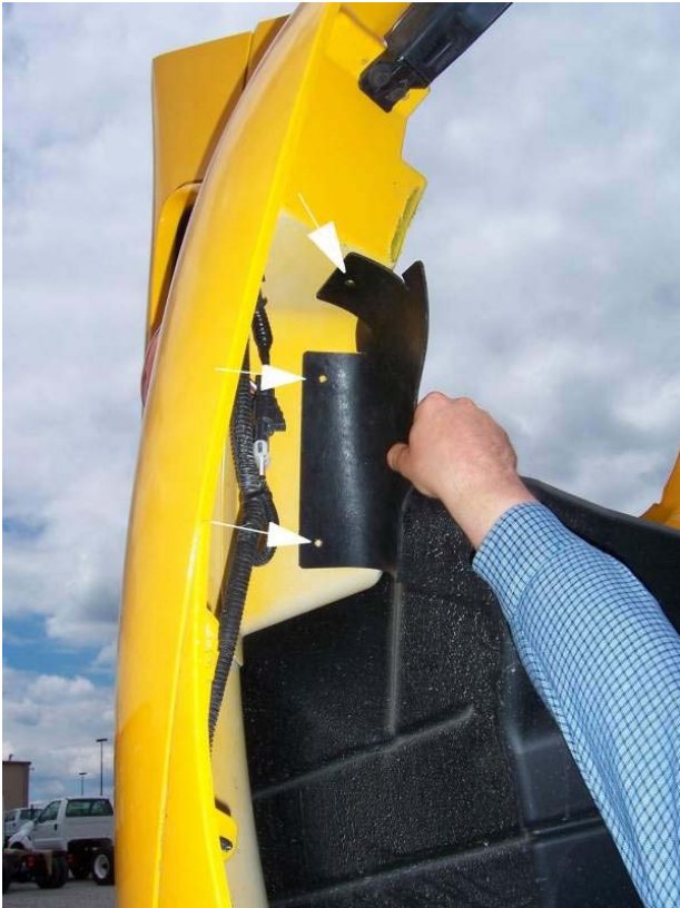
Figure 7 Hold Rubber Splash Deflector to Locate and Mark Mounting Holes
