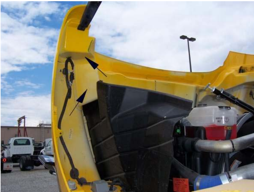
Figure 5 Rear Hood Reinforcement Area (see Arrows)
