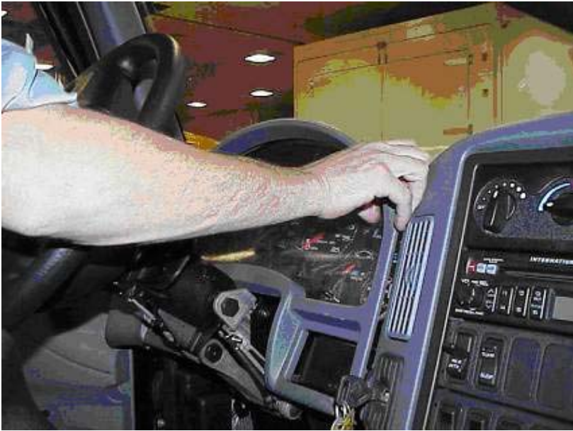
Figure 2 Remove Cluster Dash Trim Panel
