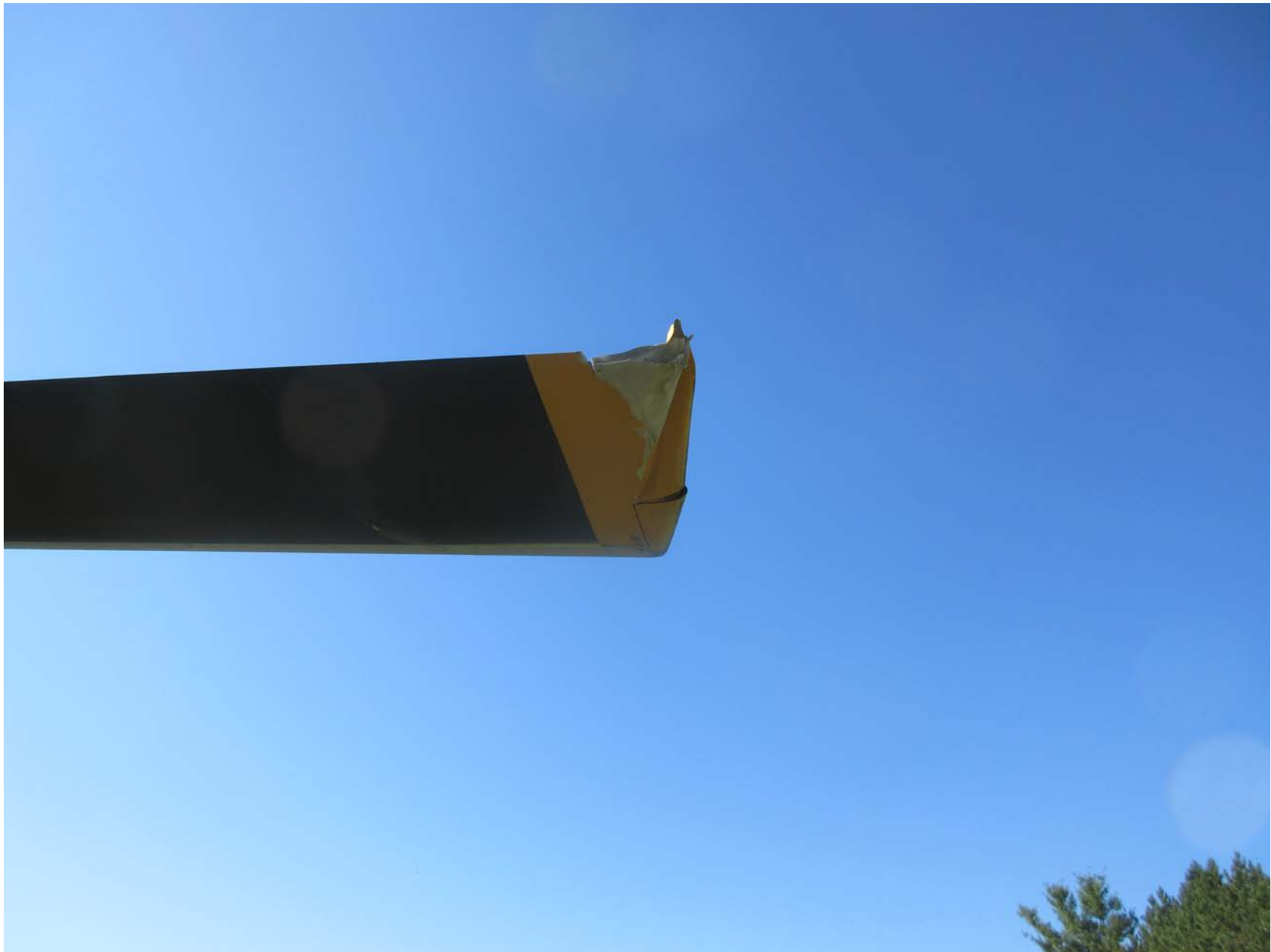
Photo 6 – Damaged main rotor blade tip (FAA photo)
