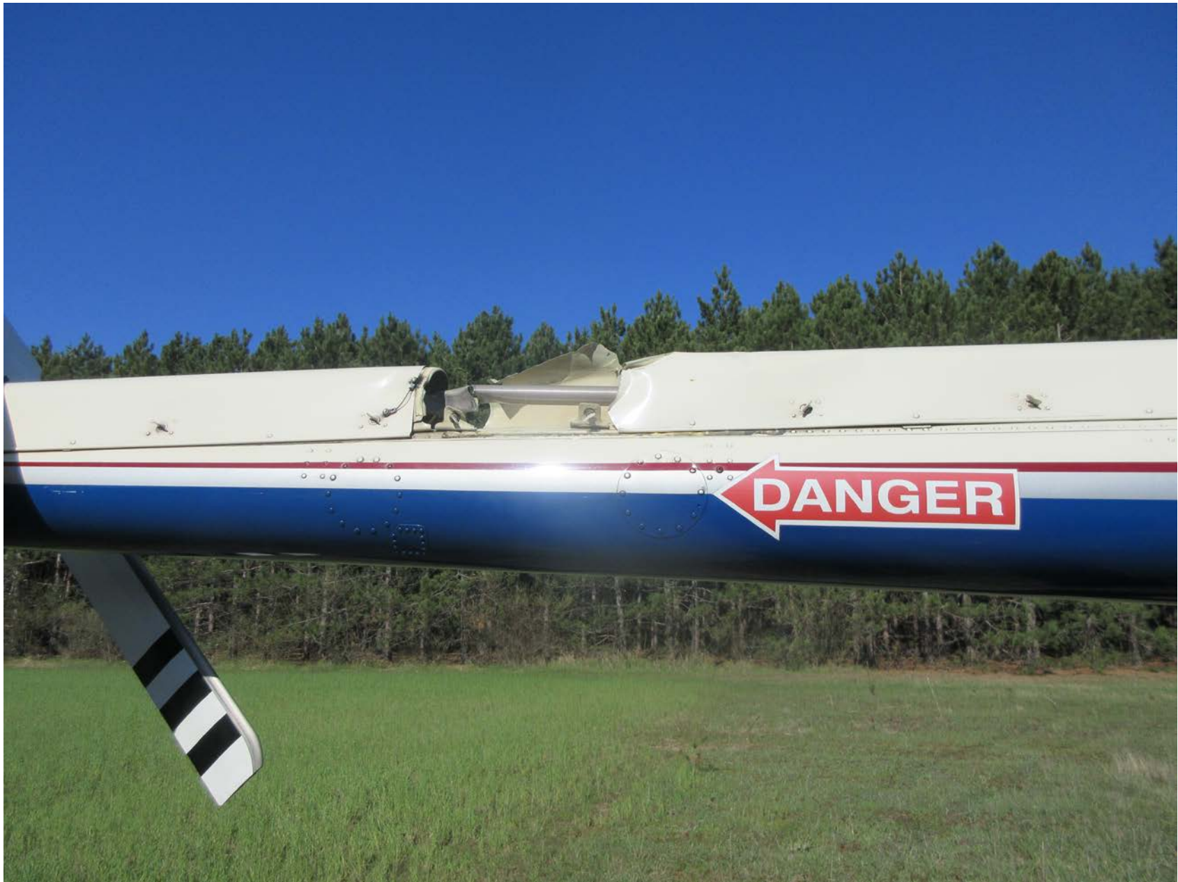
Photo 4 - Tail boom covering torn away, exposing severed tail rotor driveshaft (FAA photo)
