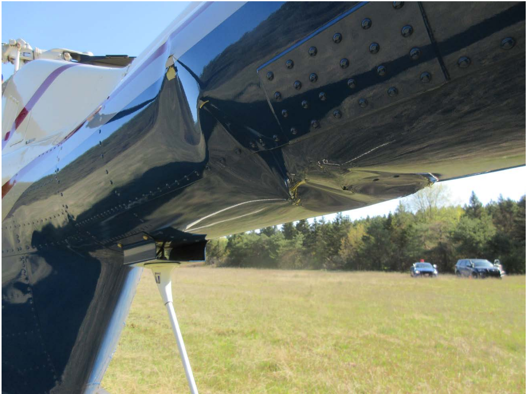
Photo 5 – Impact Buckling on bottom of tail boom (FAA photo)
