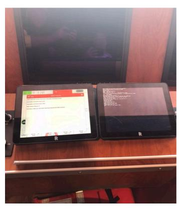
Screen A with SD card from B, and Screen B with SD card from A. Rebooting issue has followed the SD card.
