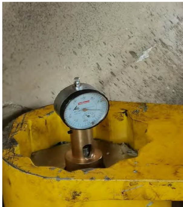
Measuring bolt stretch
