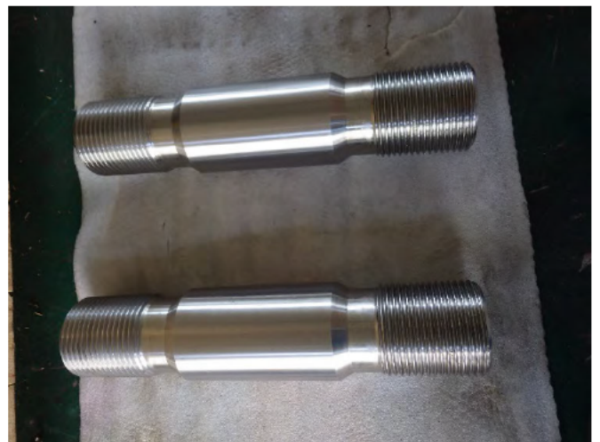
Coupling bolts view after grinding
