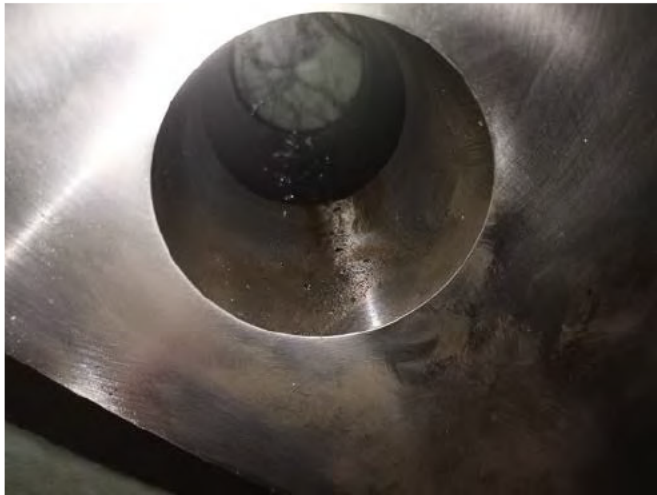
Coupling hole view before boring
