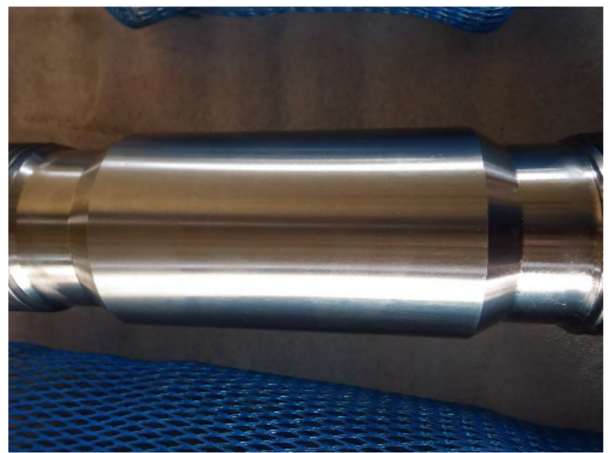
Coupling bolts contact surface view after grinding
