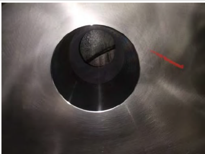
Coupling hole view after boring
