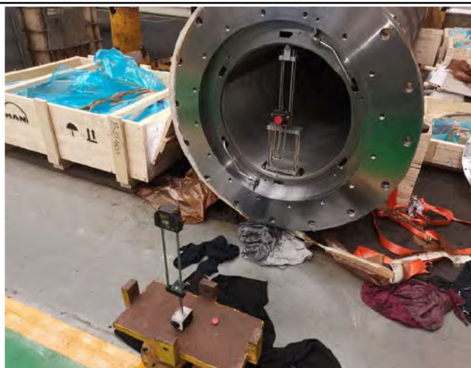
At the shipyard workshop inspection of new stern tube
