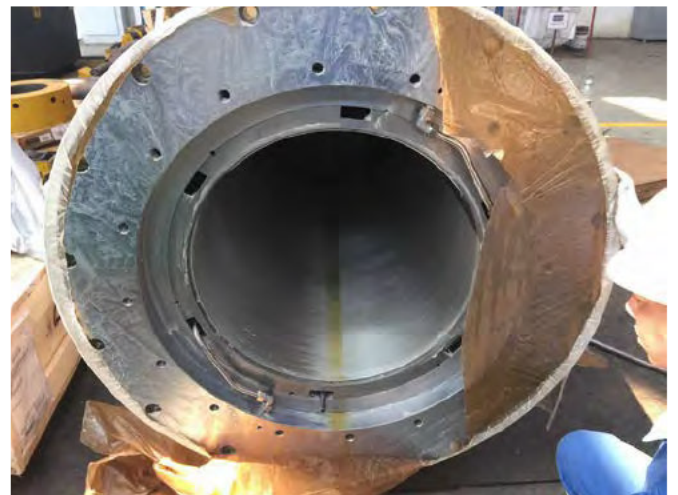
Aft stern tube bearing view
