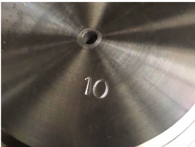
Punch 1 to 10 marking on coupling bolts end surface
