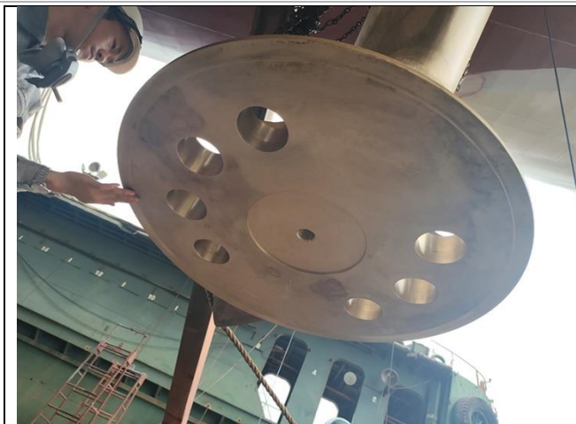
Well cleaned blade foot.
