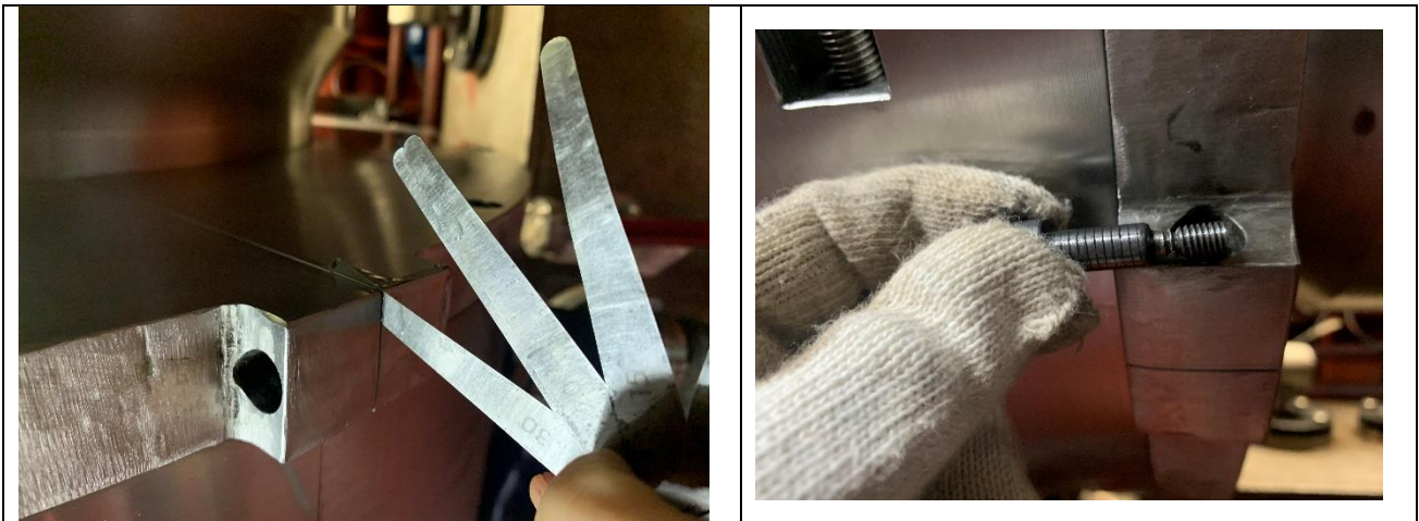
Gap between two parts was more than 0.35mm, and broken alignment bolt
