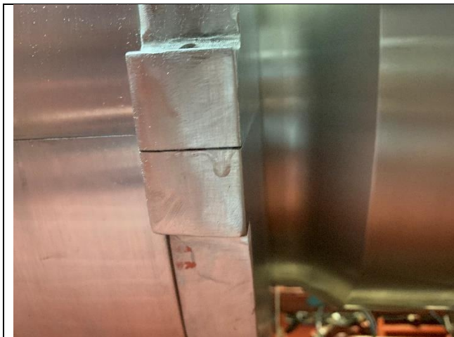
Oil leaking from end cover contacting area
