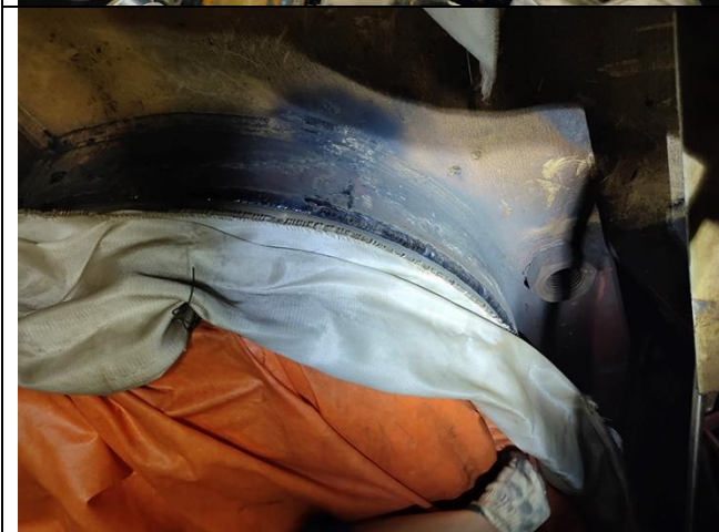
Cross welded the welding flange onto hull boss.
