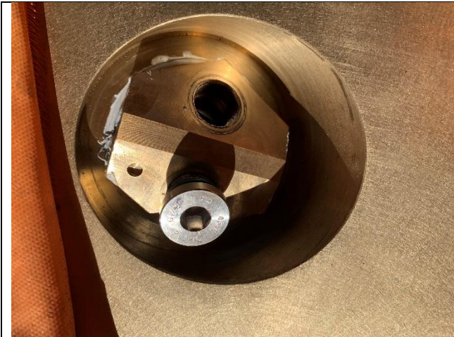
Filled hub oil and pressure tested
