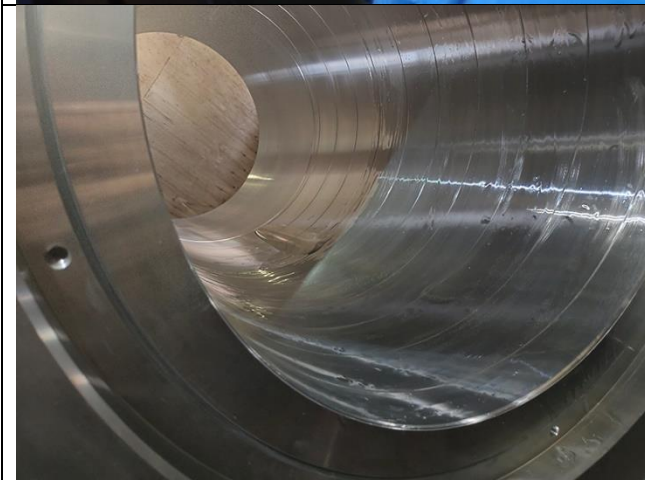
Lubricated coupling flange with lubrication oil.
