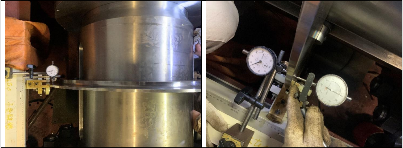
Feedback ring alignment checked and adjusted
