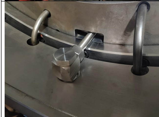
Connected banjo coupling of sampling pipe with LOCKTITE 572.
