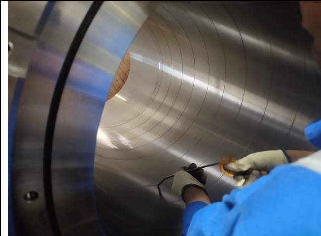
Well cleaned coupling flange inside.
