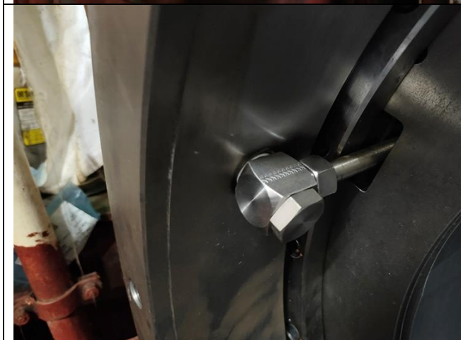
Assembled oil box and connected banjo couplings of after seal pipes with LOCTITE 572.
