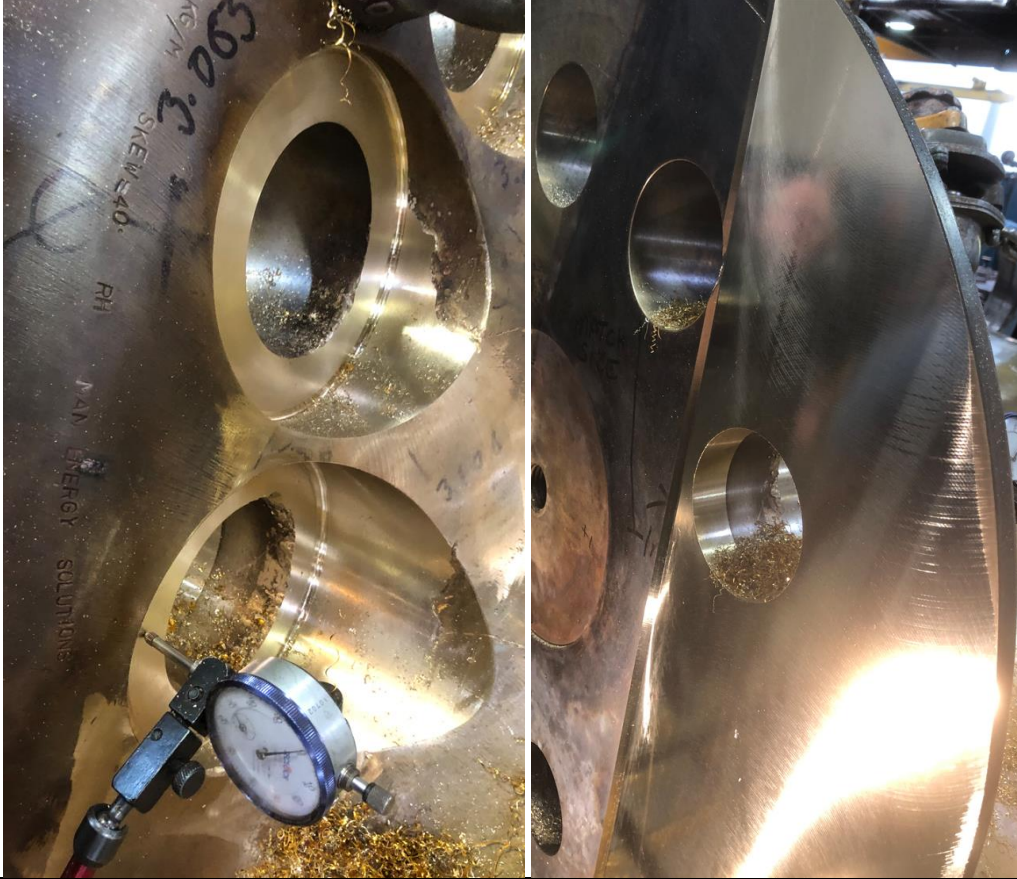
Blade 2# screws holes 6 - 7 after machining and with radius 3mm.
