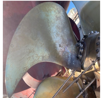
Repaired #2 blade installed
