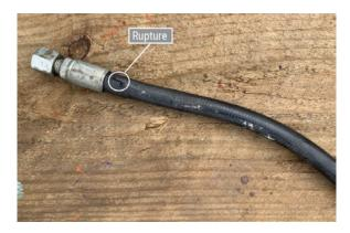
The ruptured hose was configured similar to the below photograph of the replacement hose. The hose burst was near the coupling, approximately facing the 1 o'clock position.
