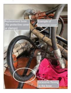
Additionally photographs of the damage hose are attached. I currently do not possess the specs on the crimp OD or fitting other than what is show in the photographs.
