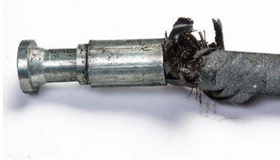
Hose Burst at Coupling
