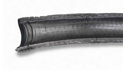
Hose Tube Failure
