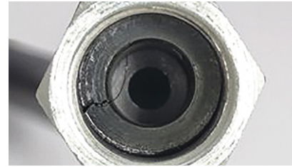
Mated Angle Seat Cracks
