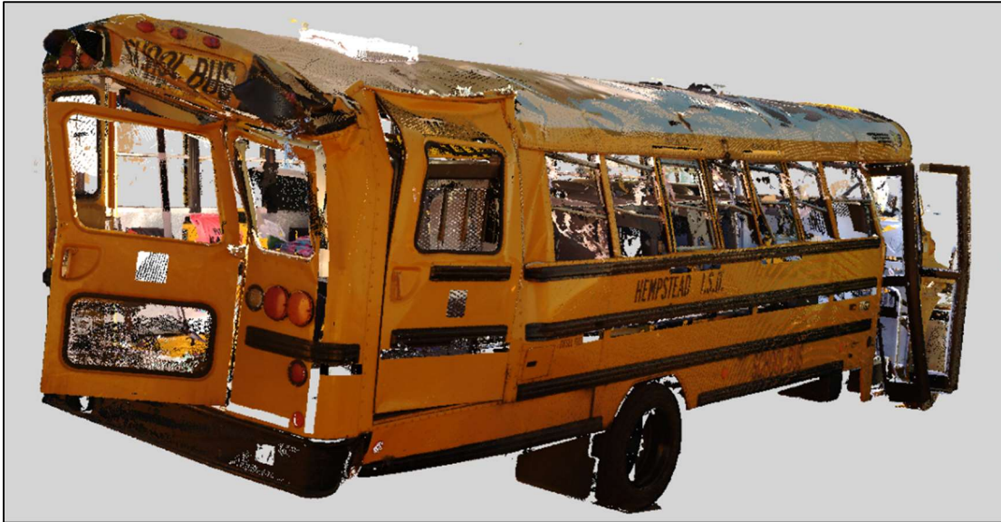
Figure 8: Screen capture image of the 3D point cloud rendering of the involved bus as observed from the right rear of the vehicle.
