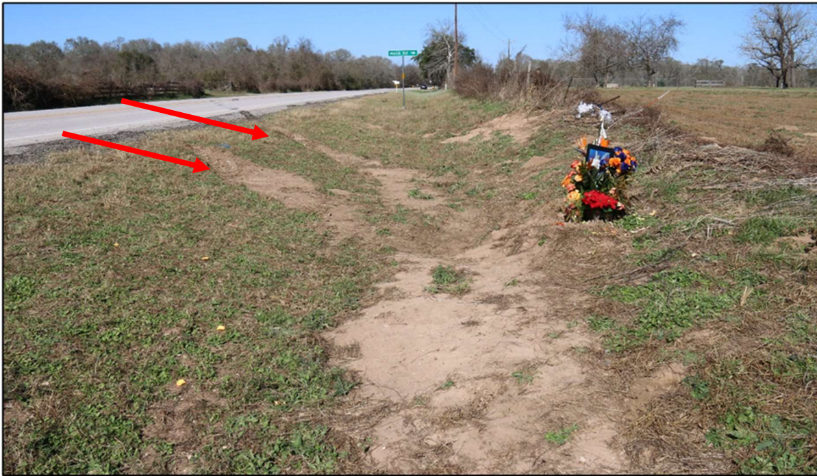
Figure 4: Photograph depicting northward view of east roadside adjacent the northbound travel lane where the school departed the highway and overturned. Soil furrows (indicated by red arrows) from the bus tires are visible.
