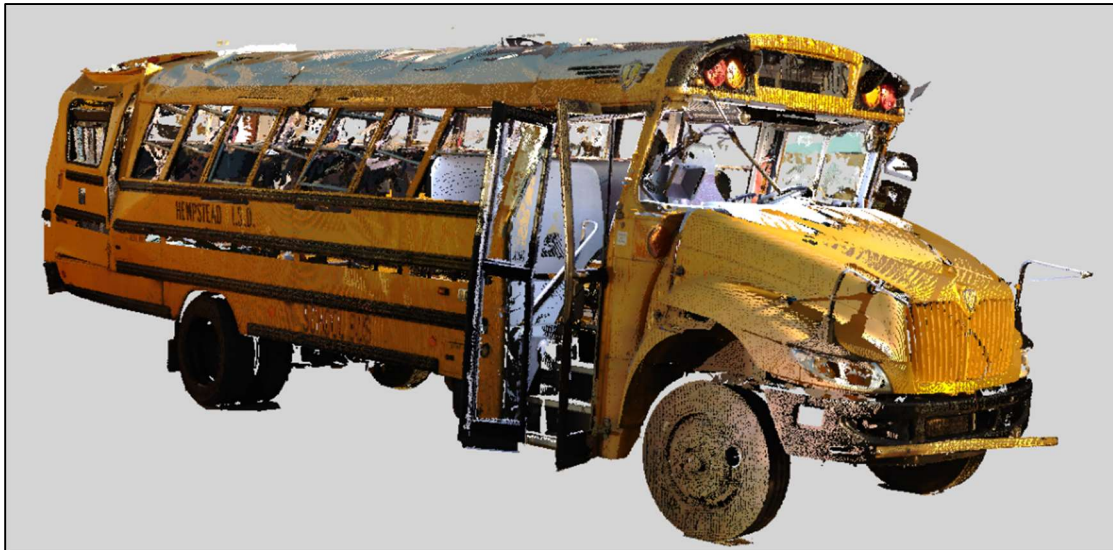
Figure 7: Screen capture image of the 3D point cloud rendering of the involved bus as observed from the right front of the vehicle.
