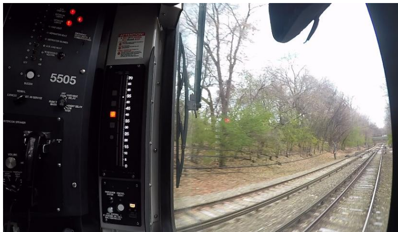
Figure #3: Test Run #1 – Speed when stop code command was received from signal system
