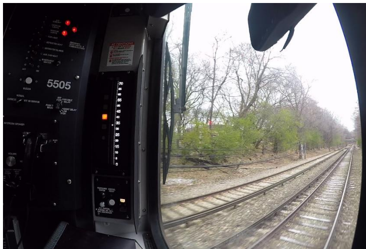
Figure #17: Test Run #5 – Speed when stop code command was received from signal system
