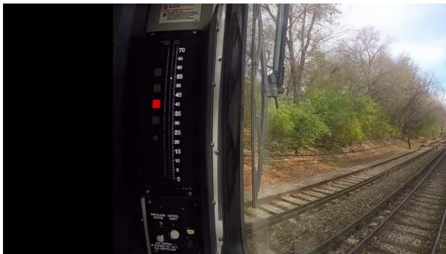
Figure #7: Test Run #3 – Speed when stop code command was received from signal system
