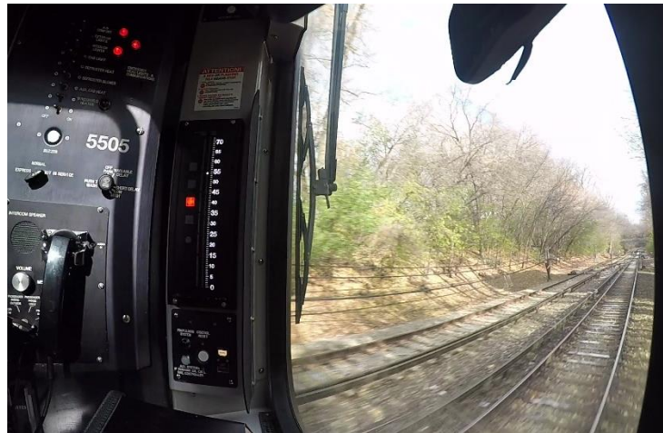
Figure #19: Test Run #6 – Speed when stop code command was received from signal system
