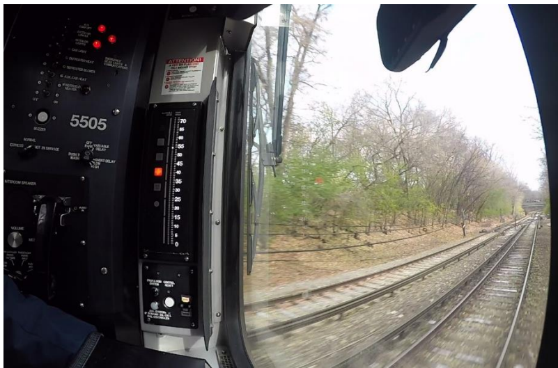
Figure #9: Test Run #3 – Speed when stop code command was received from signal system
