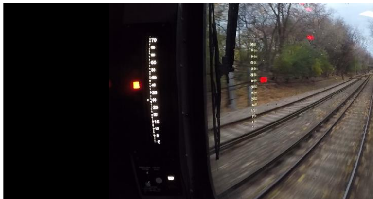
Figure #4: Test Run #1 – Speed when stop code command was received from signal system
