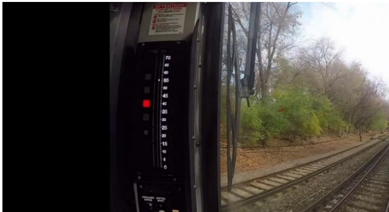
Figure #3: Test Run #1 – Speed when stop code command was received from signal system
