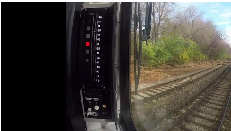
Figure #5: Test Run #2 – Speed when stop code command was received from signal system
