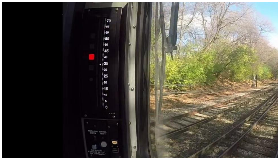
Figure #11: Test Run #4 – Speed when stop code command was received from signal system
