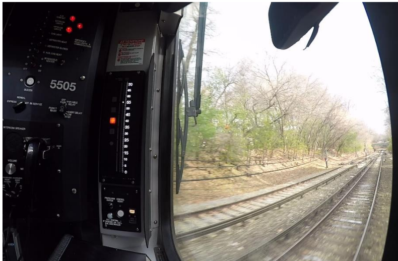
Figure #13: Test Run #3A – Speed when stop code command was received from signal system
