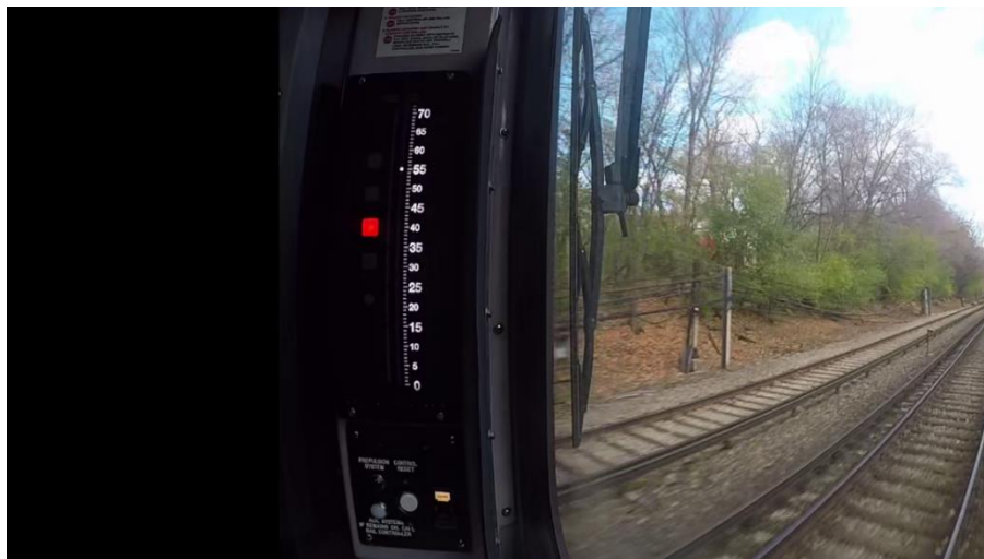
Figure #15: Test Run #6 – Speed when stop code command was received from signal system
