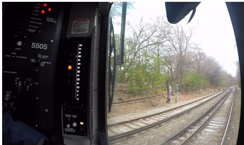
Figure #11: Test Run #3-Take 2 – Speed when stop code command was received from signal
