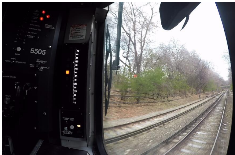
Figure #25: Test Run #9 – Speed when stop code command was received from signal system
