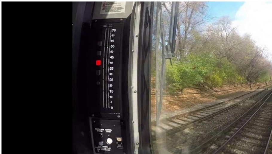
Figure #9: Test Run #3A – Speed when stop code command was received from signal system
