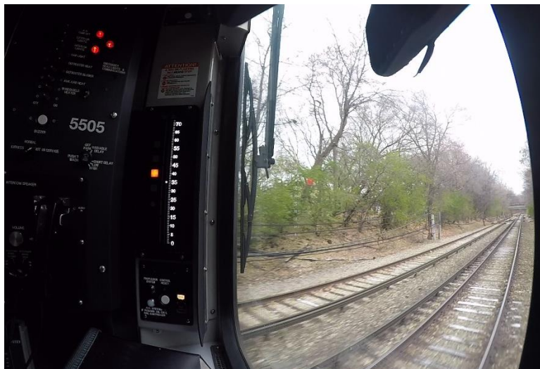
Figure #15: Test Run #4 – Speed when stop code command was received from signal system
