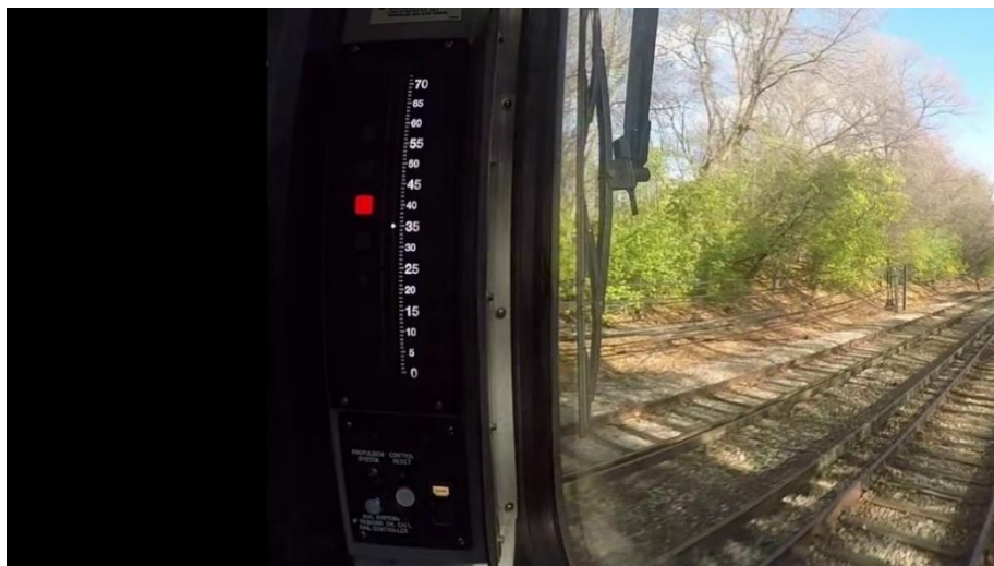
Figure #13: Test Run #5 – Speed when stop code command was received from signal system
