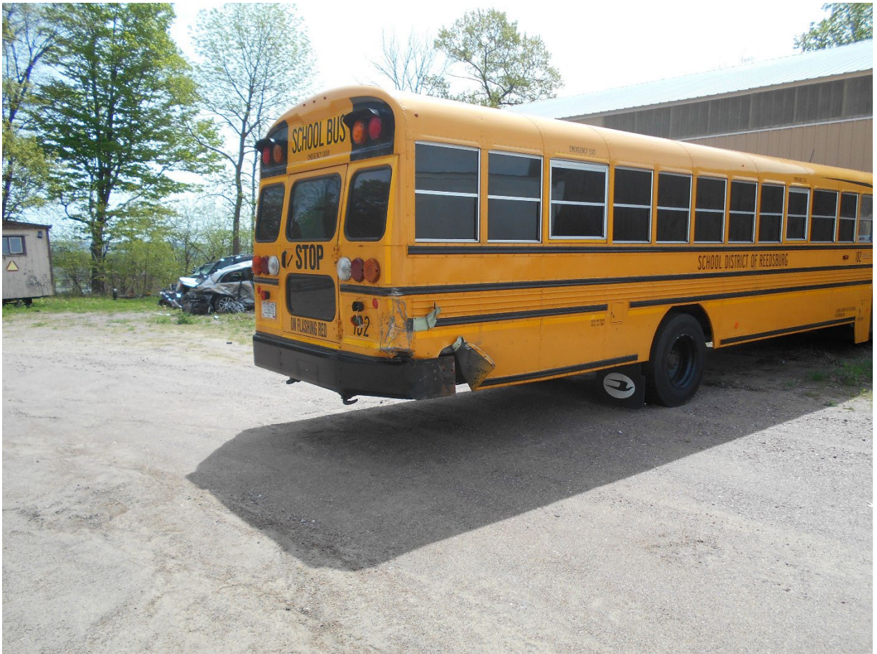
Photo 3: Photo of damage to the rear of bus #182.( Source: NTSB)
