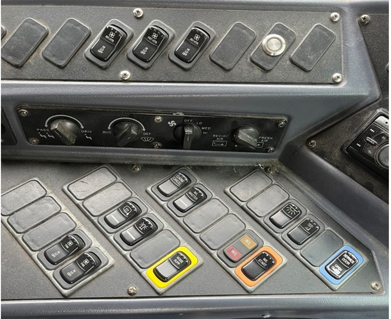
PHOTO 2: This is a photo of the warning lights and stop arm and door switch on Reedsburg Bus #182 (Source: NTSB)
